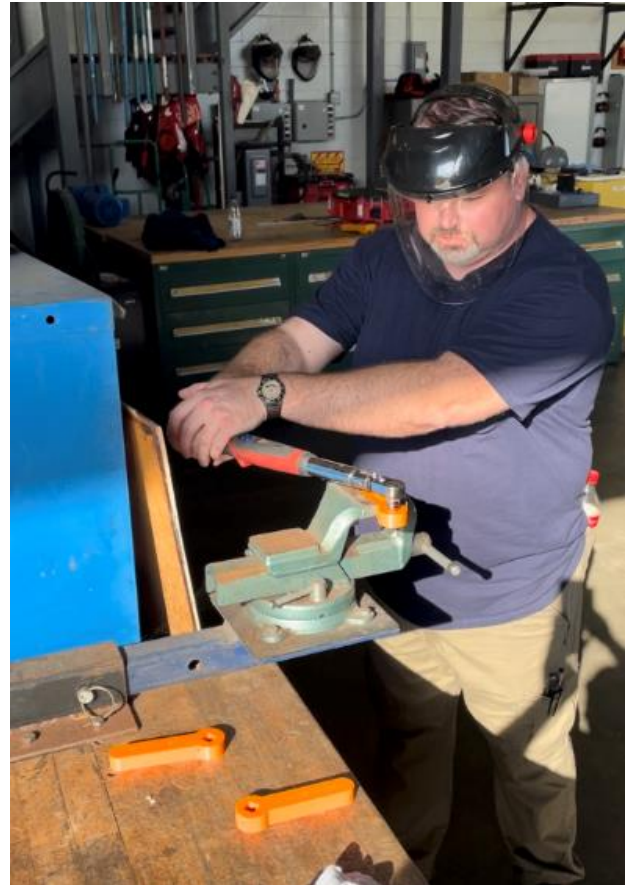
Figure 3. IPF member testing the ultimate strength of a part. (Source: U.S. Coast Guard)
