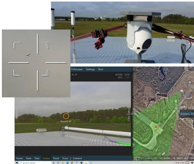
Figure 2. The sensor temporarily mounted for ground testing. (Source: U.S. Coast Guard)
