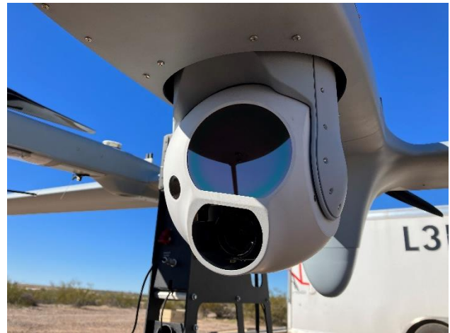
Figure 1. HD80-MV 36X mounted on L3Harris FVR-90. (Source: U.S. Coast Guard)
