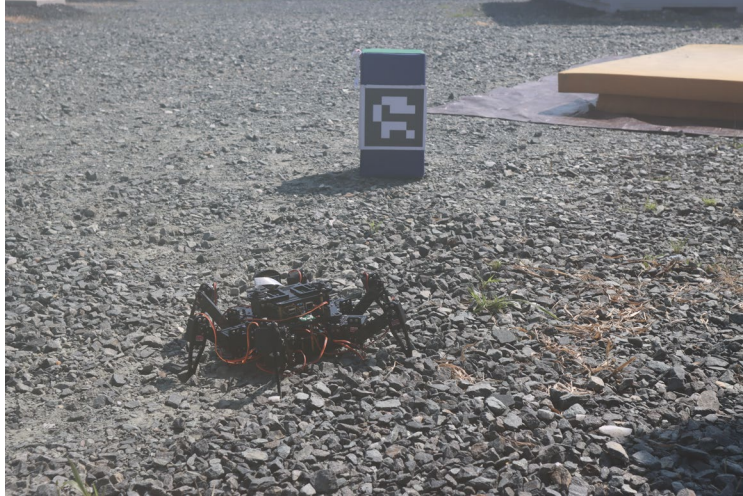
Fig. 5 Hexapod robot performs the navigation task of locating and moving toward an Aruco marker
