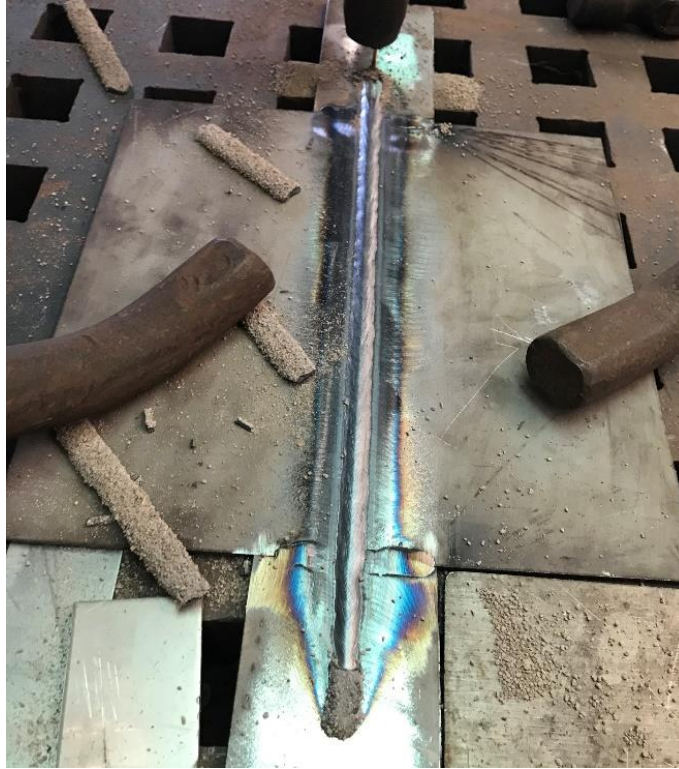
Figure 5. Representative butt joint weldment of HY-100 material investigated for plate, weld, and HAZ microstructures. The tee joint configuration was not imaged prior to cross-sectioning, but the shape and size is representative of the previous marine steel alloy efforts.
