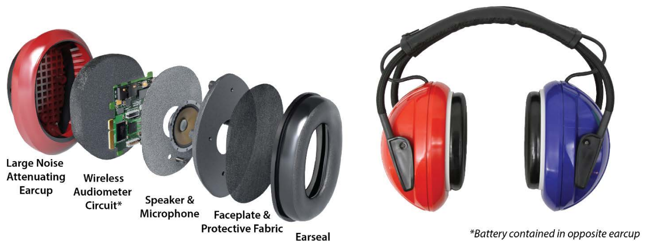
Figure 2. Composition of the wireless audiometric headset. (Meinke et al., 2017). Image source: Creare®. Used with permission.
