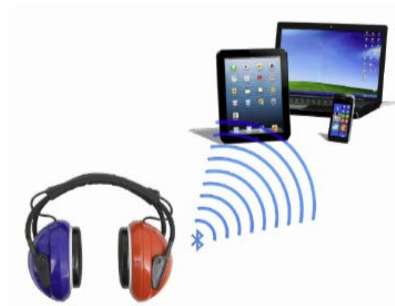
Figure 1. The Wireless Automated Hearing-Test System (WAHTS) was created by Creare® to assess hearing without the need for a soundproof room or audiometric booth. The system consists of a calibrated headset and a tablet or PC computer that administers the tests. The headset provides ambient noise attenuation and serves as the “boothless” aspect of the system. (Creare®, 2019). Image source: Edare Inc. Used with permission.
