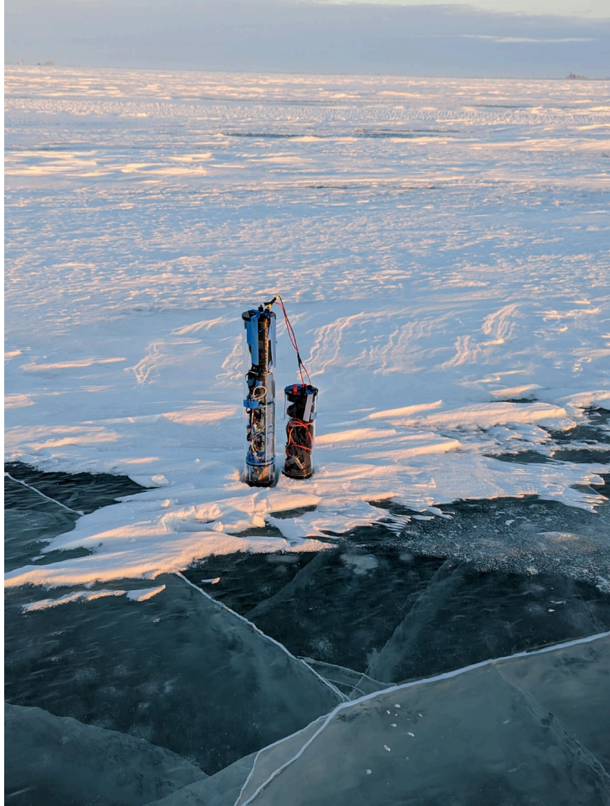
Figure 5: Cryophone and external battery capsule frozen into Lake Colleen.
