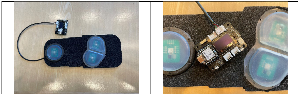
Figure 2. ORToS CAMWalker boot insole with the nRF52840 microcontroller evaluation assembly.
