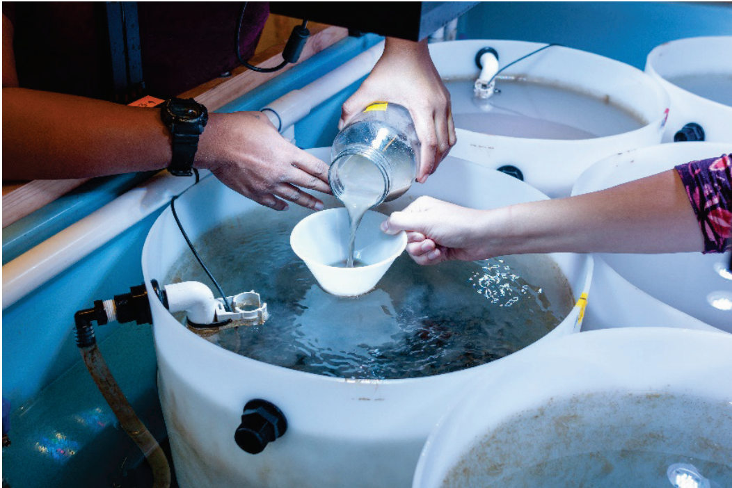
Figure 12. Procedure for adding fine-grain sediment to test tanks (Photo: Justin Wilkens).
