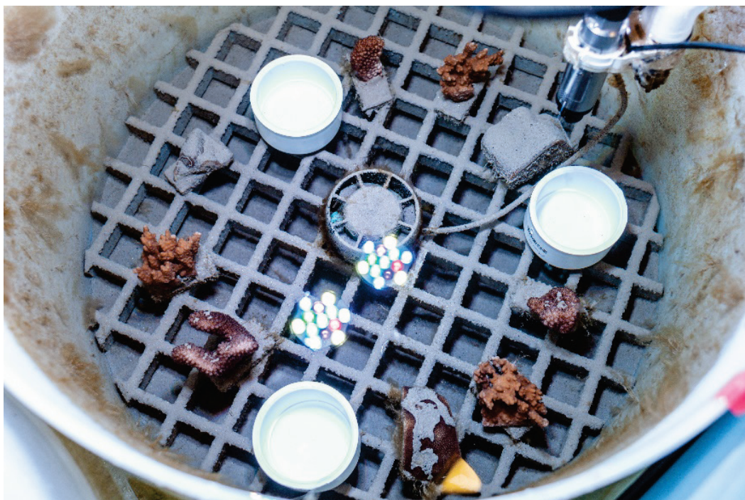
Figure 14. Photo of three sediment traps (PVC cap with a surface area of 28.6 \text{ cm}^2 ) placed on the bottom grate near corals prior to a sediment dose (Photo: Justin Wilkens).
