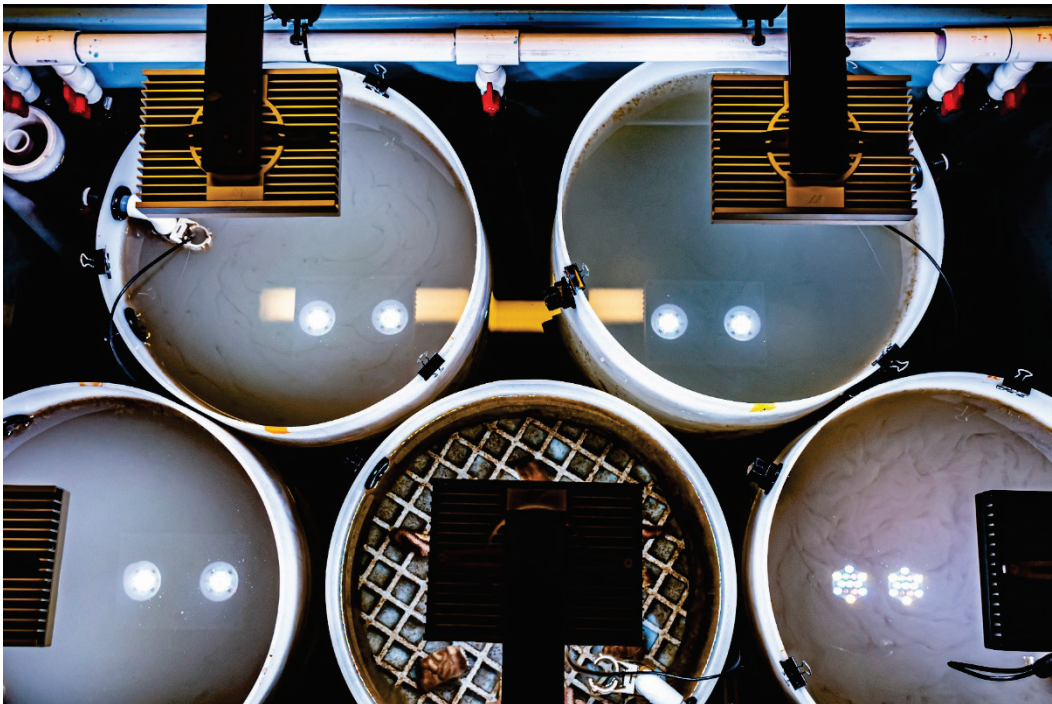
Figure 20. Photo taken during 15 min sedimentation period in one module of test tanks dosed with fine grain sediment to create sedimentation concentrations of 0-control, 6, 30, and 60 mg cm -2 . Clockwise from top left: 60, 6, 60 0 (control), and 30 mg cm -2 (Photo: Justin Wilkens).
