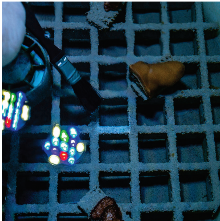
Figure 26. The sediment on the bottom grate is brushed away to highlight sediment coverage after second dose to create sedimentation concentration of 60 mg cm -2 with fine grain sediment (photo: Justin Wilkens).
