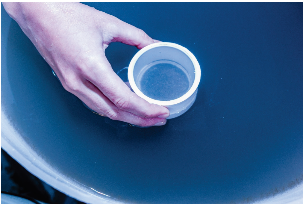
Figure 15. A sediment trap (PVC cap with a surface area of 28.6 \text{ cm}^2 ) removed from a test tank after the 15 min sedimentation period following sediment dosing. The contents were used to determine the 15 min net sedimentation concentration ( \text{mg cm}^{-2} ) (Photo: Justin Wilkens).
