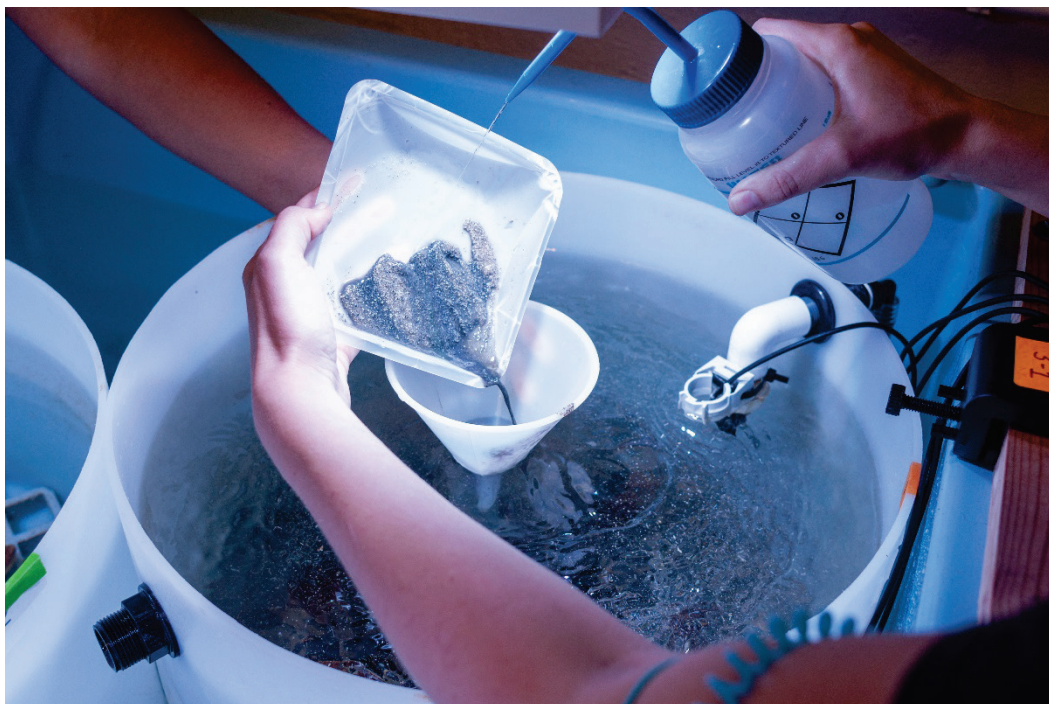
Figure 13. Procedure for adding coarse-grain sediment to test tanks (Photo: Justin Wilkens).
