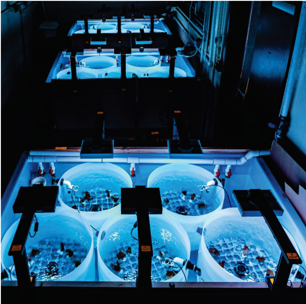
Figure 6. The exposure system within a temperature and light-controlled area at the Kewalo Marine Laboratory. The system consisted of three rectangular water baths each with five partially submerged flow through circular test tanks. Each tank was filled with 55 L of 5 \mu m filtered seawater introduced continuously through a diffused outlet near the top of the tank (Photo: Justin Wilkens).
