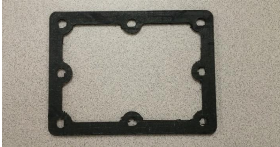
Figure 13. 3D printed gasket (Author Photo).
