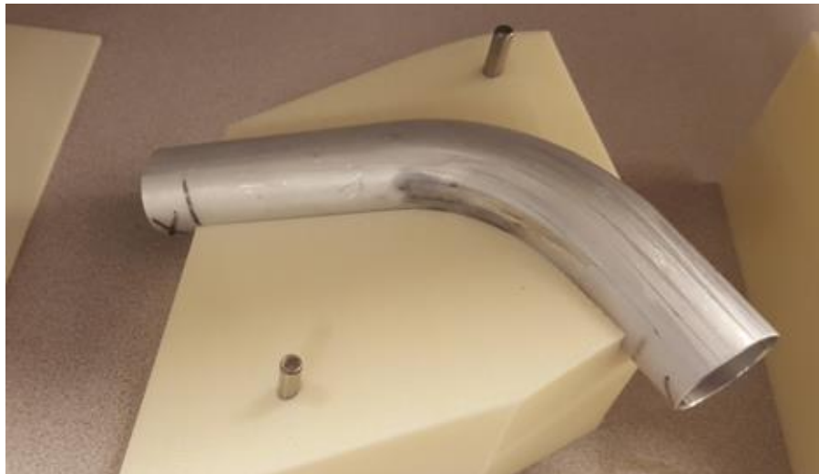
Figure 7. 3D Printed band saw guide for H-65 fuel tube (ALC Photo).
