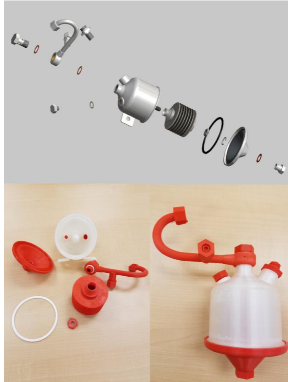
Figure 16. Disk pack filter model and 3D printed parts (Photo: Ryan Delbridge, USCG).
