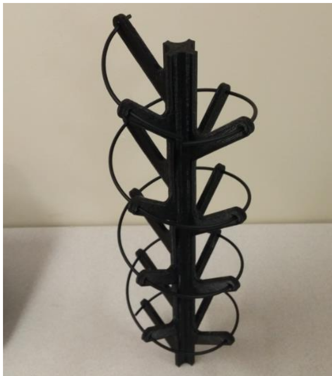
Figure 12. 3D printed Helical Antenna (Author Photo).
