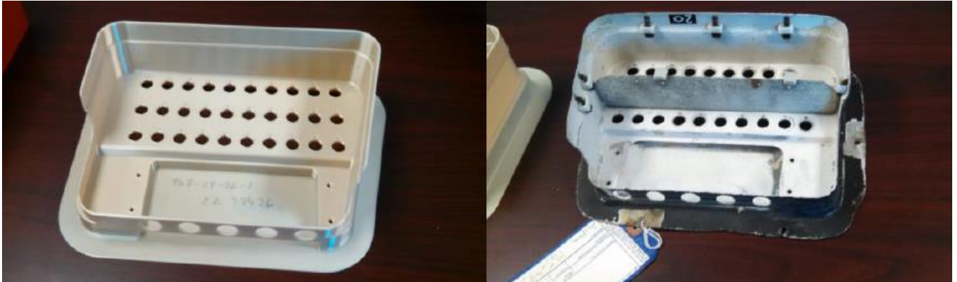
Figure 6. ALC's 3D Printed circuit panel (left) and original part (right) (Photo: William Bryan, CG-444).
