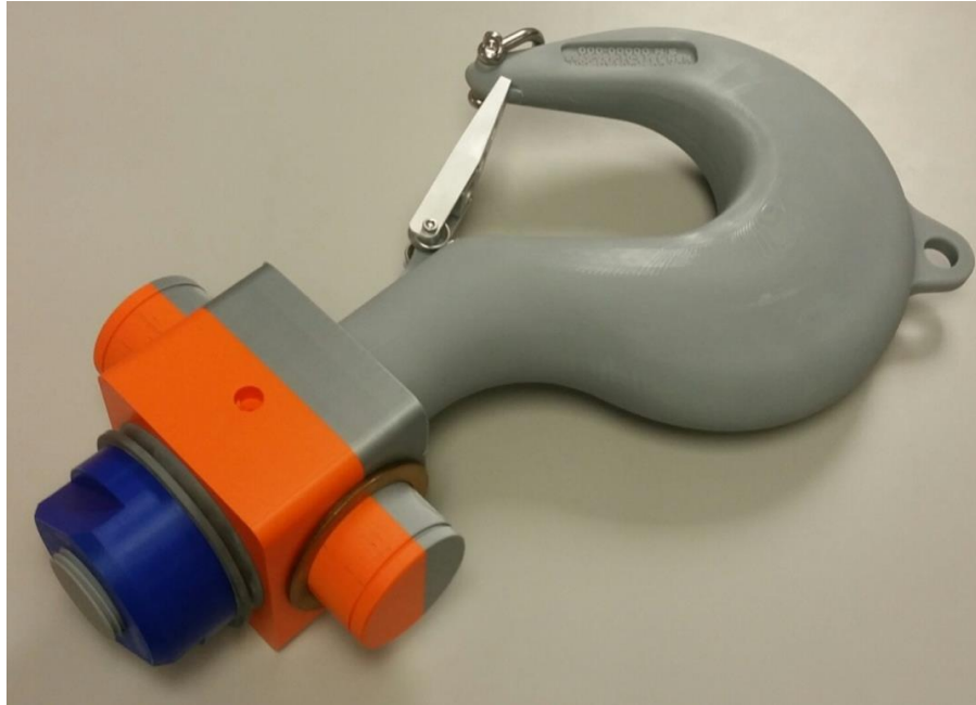
Figure 20. Full scale crane lifting block subassembly (Photo: Ryan Roberts, SFLC).
