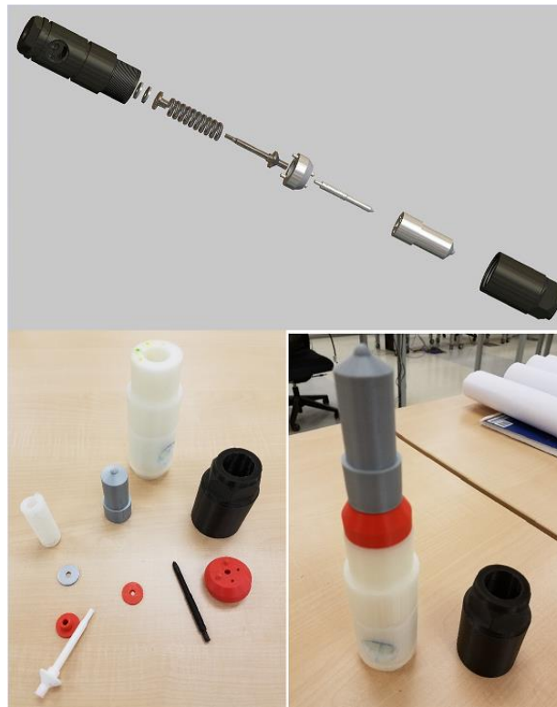
Figure 15. Fuel injector model and 3D printed parts (Photo: Ryan Delbridge, USCG).
