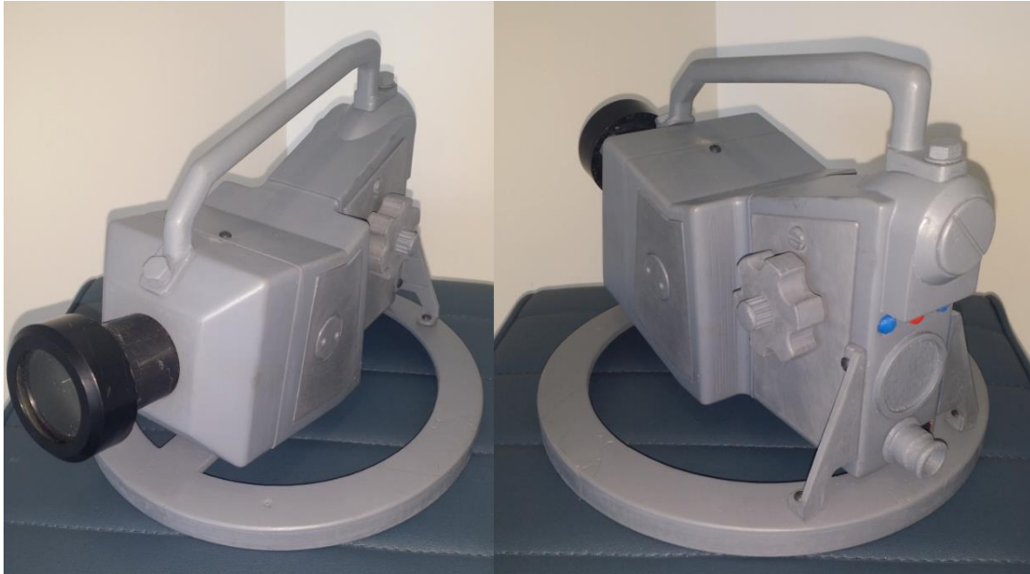
Figure 17. 3D printed simulation alidade box (Photo: Brian Dooley, USCG).
