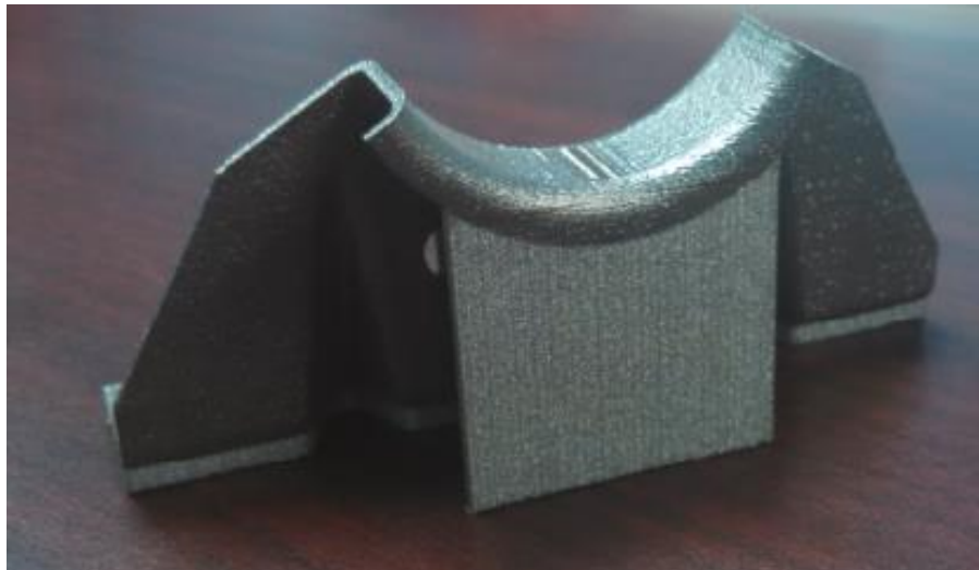
Figure 4. 3D printed metal flange showing support structure (Photo: William Bryan, CG-444).
