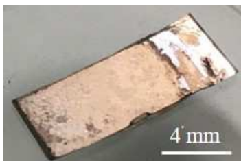
Figure 8. Photograph of the Si electrode after potentiostatic electrolysis at -2.05 V in LiCl-KCl-0.24 mol%EuCl 2 melt at 723 K.
