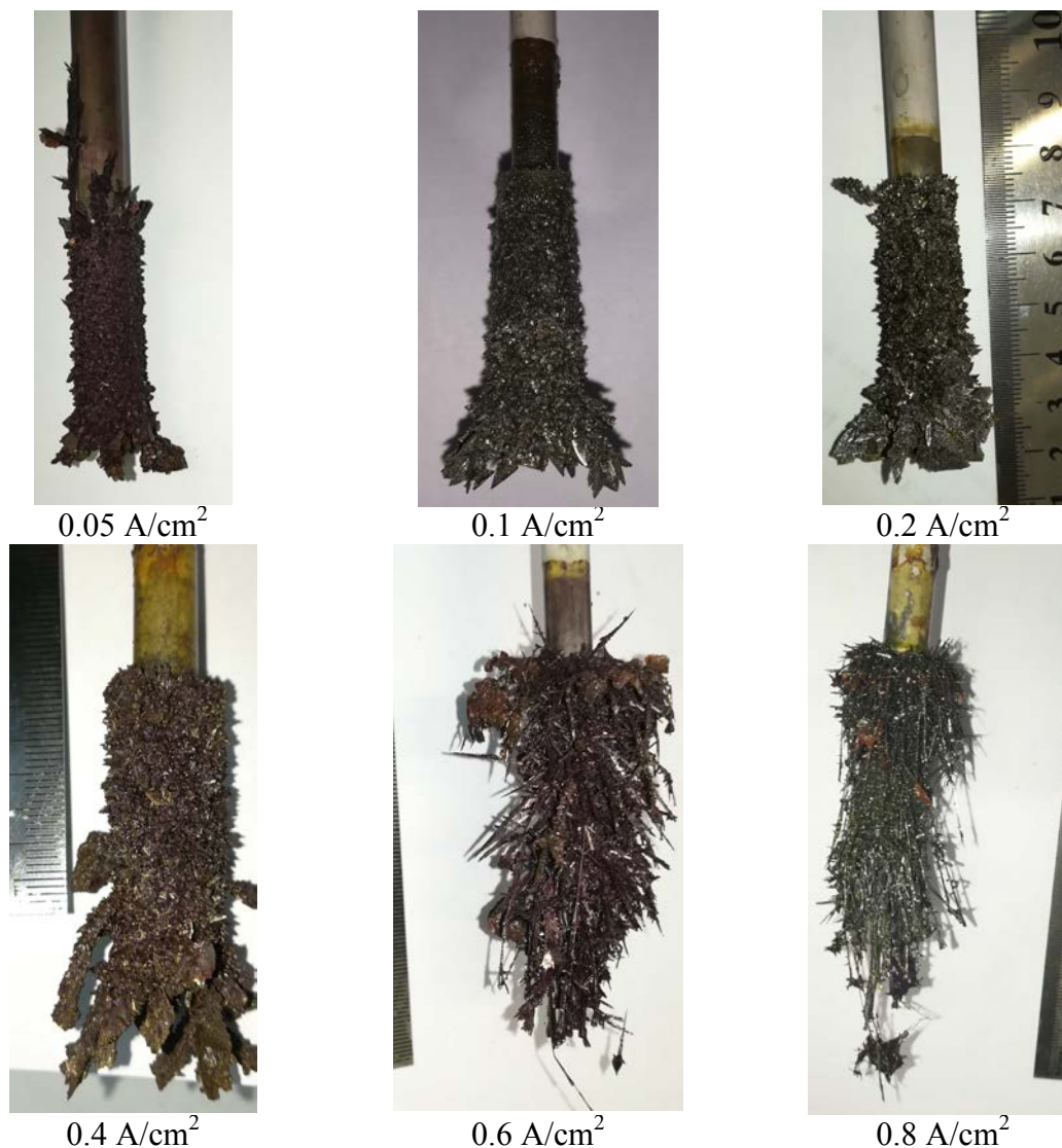
Figure 2. Cathodic deposits produced during uranium electrorefining in LiCl–KCl–UCl 3 melts at 500 °C and different cathodic current densities (shown on the graph for each sample).
