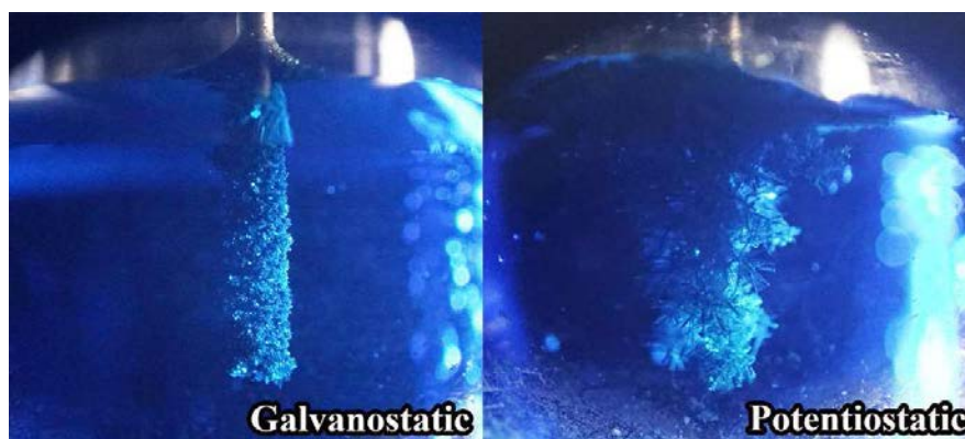
Figure 3. Images of metallic cobalt deposits on a tungsten working electrode in the molten \text{CoCl}_2\text{-LiCl-KCl} system (1 wt% \text{CoCl}_2 ) at 773K. The deposition conditions are -18 \text{ mA/cm}^2 for 1 hour galvanostatic electrodeposition and -1.6 \text{ V vs. Cl}_2/\text{Cl}^- for 30 minutes potentiostatic electrodeposition.
