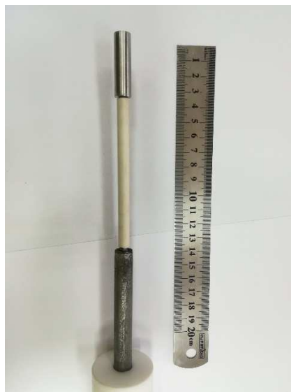
Figure 1. Cathode assembly (cathode is shown at the top).
