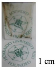
Figure 4. Photograph of the Al electroplating on Cu plate using Al mesh counter electrode in \text{EmimCl-AlCl}_3 ionic liquid at 60 ^{\circ}\text{C} without stirring (9).
