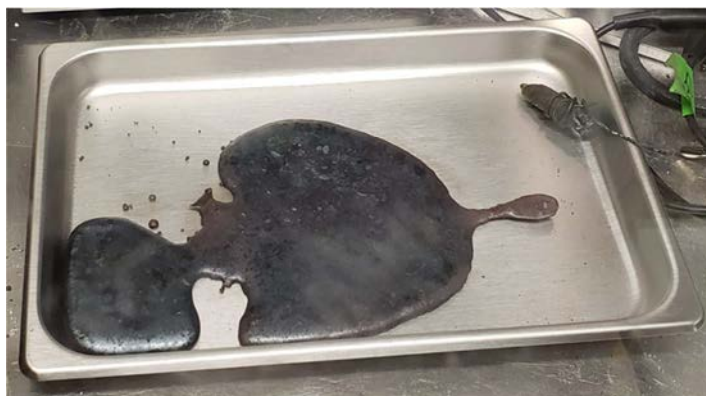
Figure 1. Image of salt batch after UCl 3 synthesis using NaCl-CaCl 2 and FeCl 3 .
