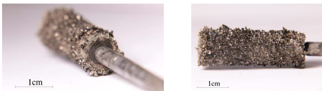
Figure 4. Uranium coating after hydrometallurgical treatment of uranium deposit produced at low cathode current densities ( 0.05 \text{ A/cm}^2 ).
