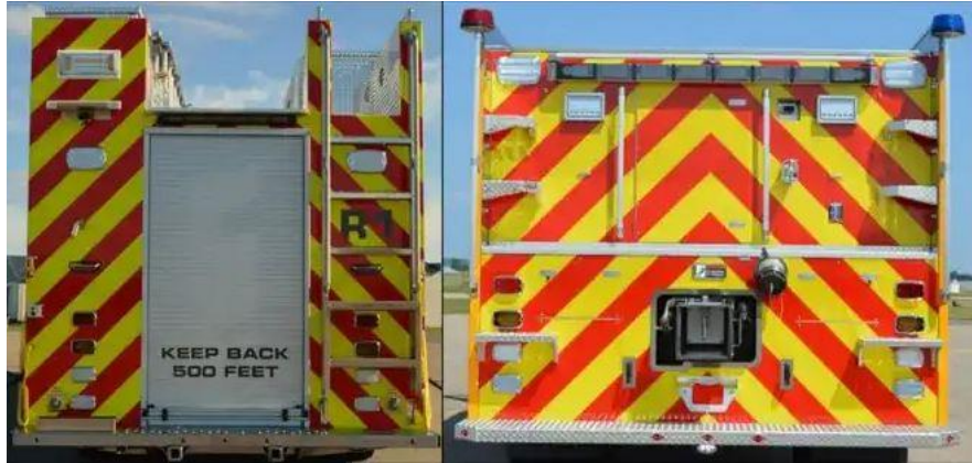
Figure 7. NFPA 1901-compliant chevron markings for fire emergency vehicles (FAMA, 2023).
