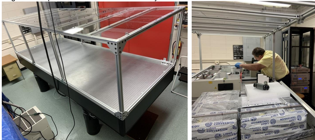
Fig.1. The RS4000 Newport optical table and the installation of the femtosecond laser system by "Spectra-Physics" Engineer.
