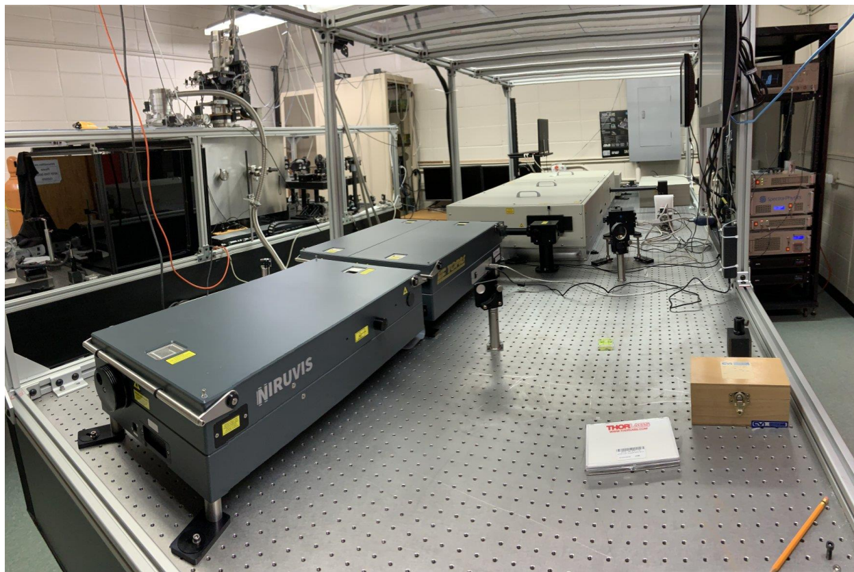
Fig.2. "Spectra-Physics" femtosecond laser system (MaiTai SP, ASCEND 60, Spitfire 35-f -1 HP ACE, Topas-U) installed in the Laboratory of Ultrafast Laser Spectroscopy, University of Puerto Rico – Mayaguez; May 2021.
