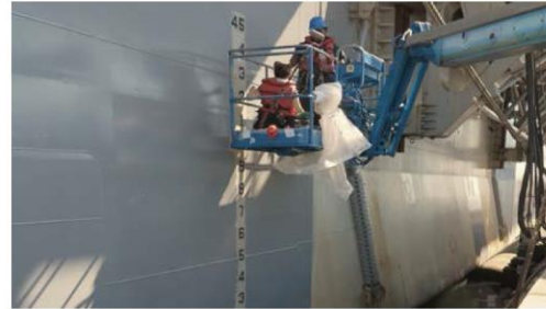
Roll application of SiloxoShield N-9999 1K by Ship's Force over a 3-year old 2K Polysiloxane on the freeboard of the USS ESSEX
