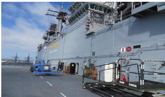
Partially finished roll and brush application of N-9999 1K by Ship's Force on the USS ESSEX
