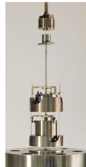
2-Sinker densimeter for p - \rho - T measurements
