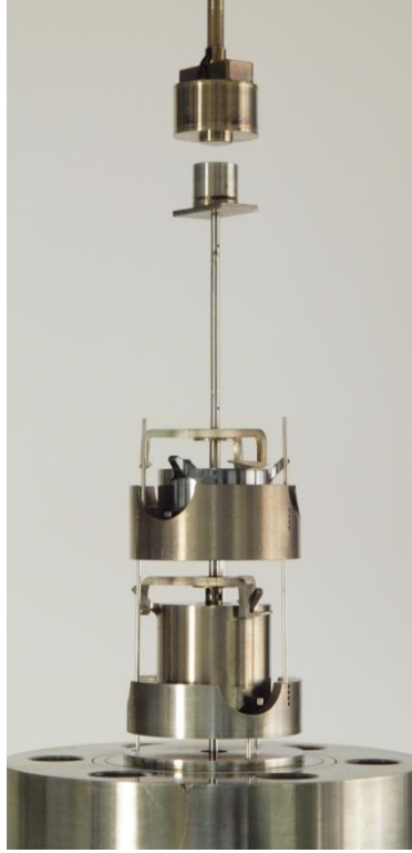
Figure A.1-3. Sinkers in the two-sinker densimeter (shown removed from the measuring cell)
