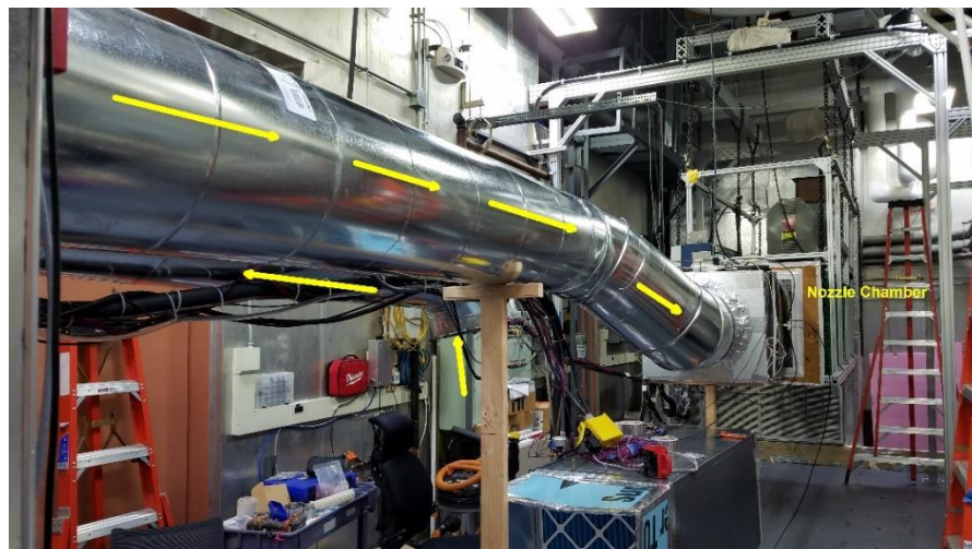
Figure 3 (Exec. Summary). Connecting ducts and nozzle chamber located in the indoor environmental chamber
