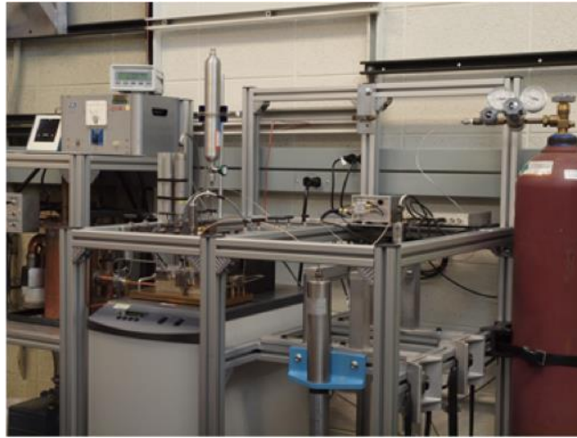
Figure A.1-4. Dual-path, pulse-echo, speed of sound instrument
