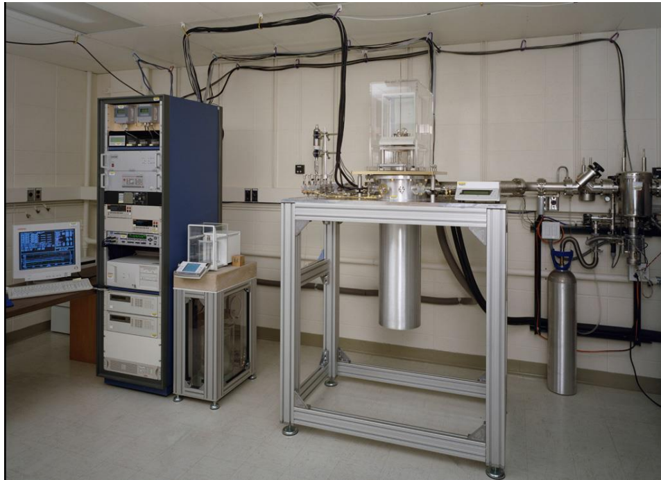
Figure A.1-2. Two-sinker densimeter
