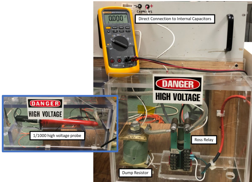
Fig. 4 Modification to the pulser module for direct shorting and monitoring of the internal capacitors through a Ross relay and external dump resistor
