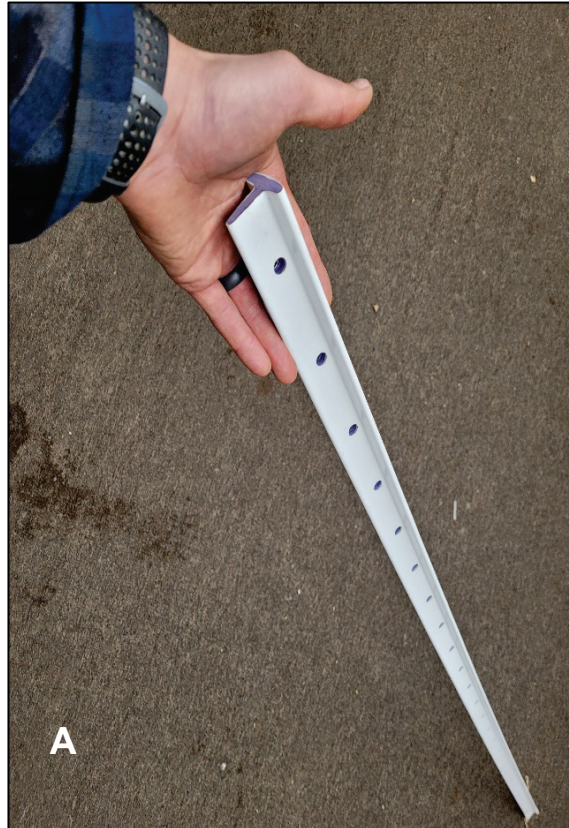
Figure 4-2. PVC T-post (A) and cross section (B), scale in inches.
