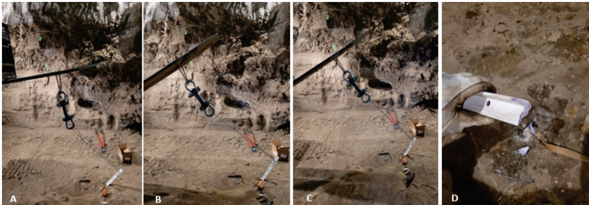
Figure 4-9. PVC in-ground flexural stress test: (A) Slack; (B) Moderate tension; (C) Heavy tension; (D) Failure.
