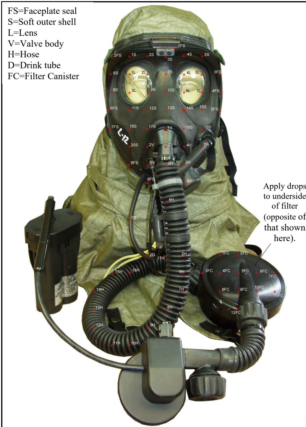
Figure A.1. Example of distilled mustard (HD) droplet contamination pattern illustration using a test item photograph for the base image.
