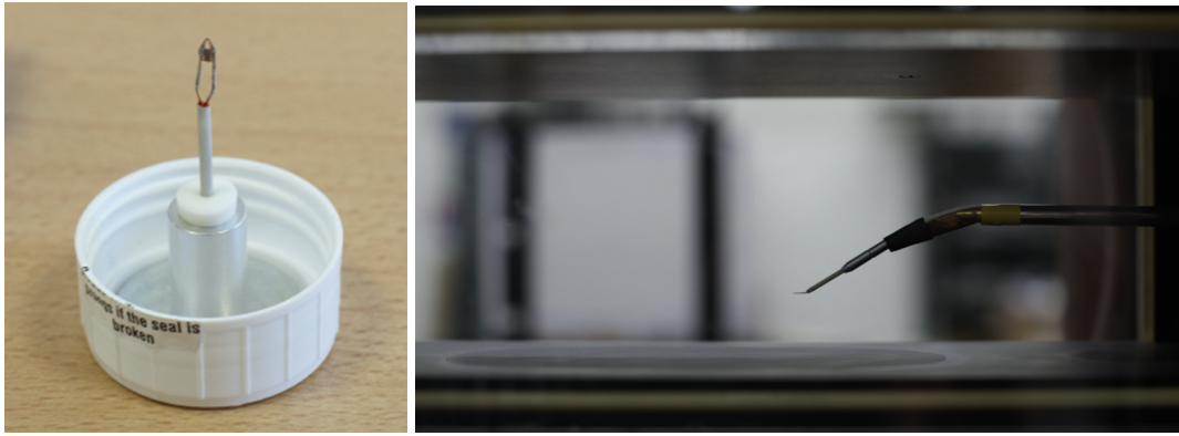
Figure 4: Probe mounted in the potential core of the flow in the supersonic wind tunnel.
