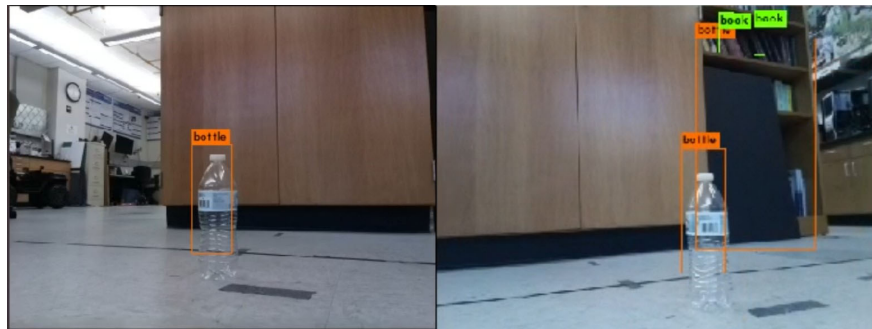
Figure 72: Image from “Mapper Agent” showing multiple detections using “darknet-ros” package for YOLO V3 from two separate agents’ viewpoints. The left image shows the view from the robot on the right looking towards the left, which shows one positive identification of a bottle. The right image shows the positive detection and one false-positive detection of a bottle on the right image.
