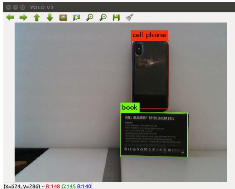
Figure 60: Identification of a cell phone using darknet_ros
