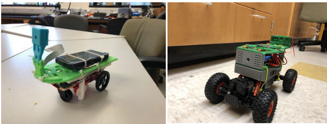
Figure 30: Photo of old model on left and new Ackerman steered platform on right with AM-L03 sensor package.
