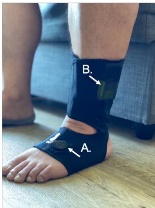
Figure 1. Participant wearing an instrumented sock, APDM prototype. The inertial sensor is located on top of the foot (A), and the main unit containing the battery in the socks is located in a second pocket just above the lateral malleolus (B). To maximize fit, the socks come in different sizes, and the Velcro attachment around the foot and ankle is adjustable to ensure a snug fit and that the sensor does not move on the foot while being worn.
