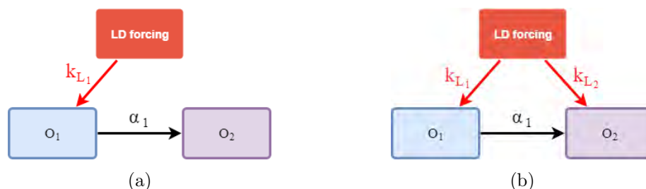
Figure 1. (a) Model with strict hierarchical coupling. (b) Semihierarchical model when both oscillators receive light input, but the light into O_2 is much weaker than the light into O_1 .
