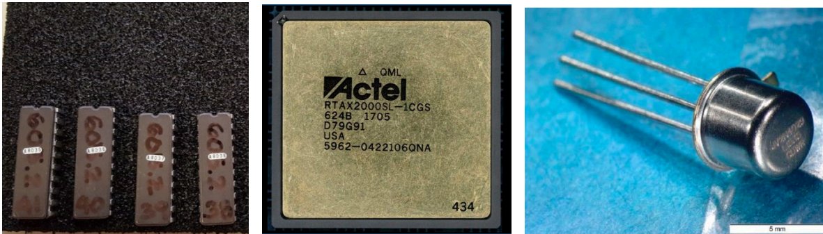
Figure 5.3. Example of a 20-pin ceramic dual in-line package (left), flat metal lid (center), and TO (can) package (right).
