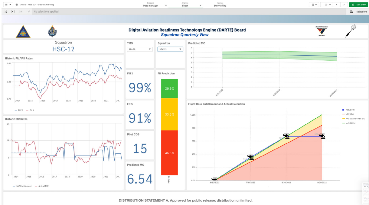
Figure 6. Squadron Quarterly View page for an MH-60 squadron. This page displays contextual information, MC predictions for the next three months, predictions of meeting quarterly FH goals, and FH execution and entitlement for the current quarter.
