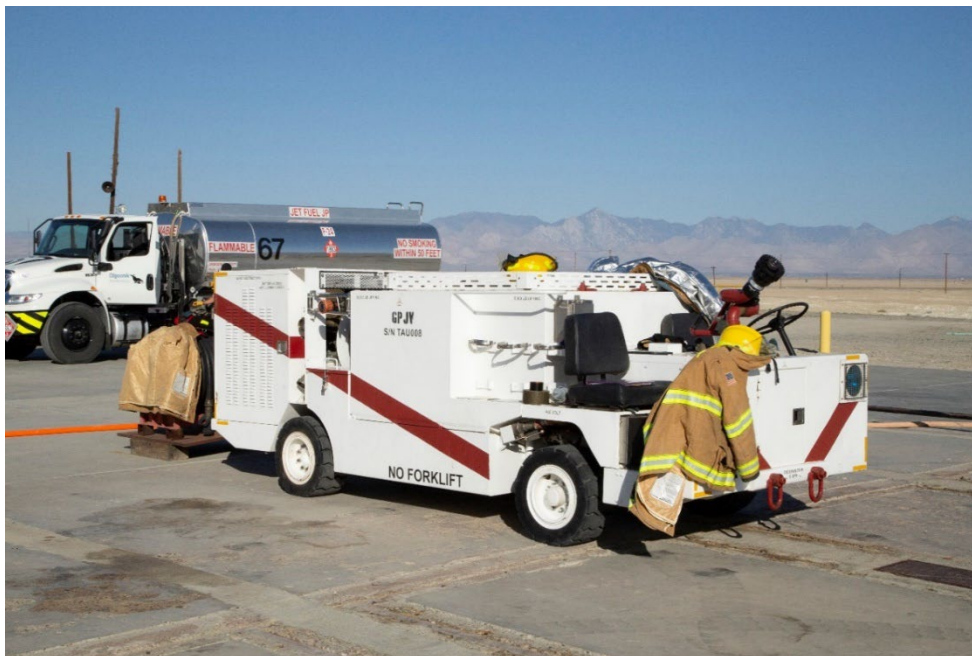
Fig. 3.4-6 – P-25A Shipboard Fire Truck (Photograph)
