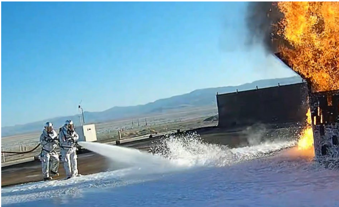
Fig. 4.6-4 – Roll-on Foam Application Pushing Toward the Debris Pile Fire
