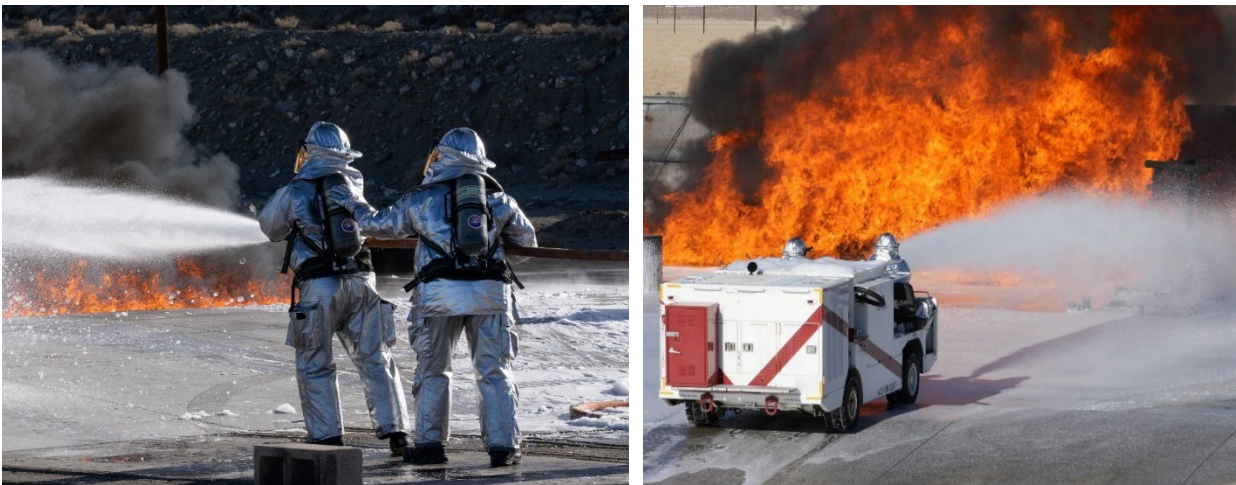
Fig. 4.5-1 – Horizontal Sweep Foam Application
