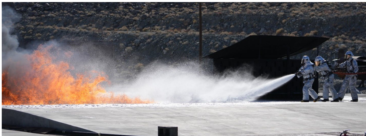
Fig. 4.5-4 – Roll-on Foam Application
