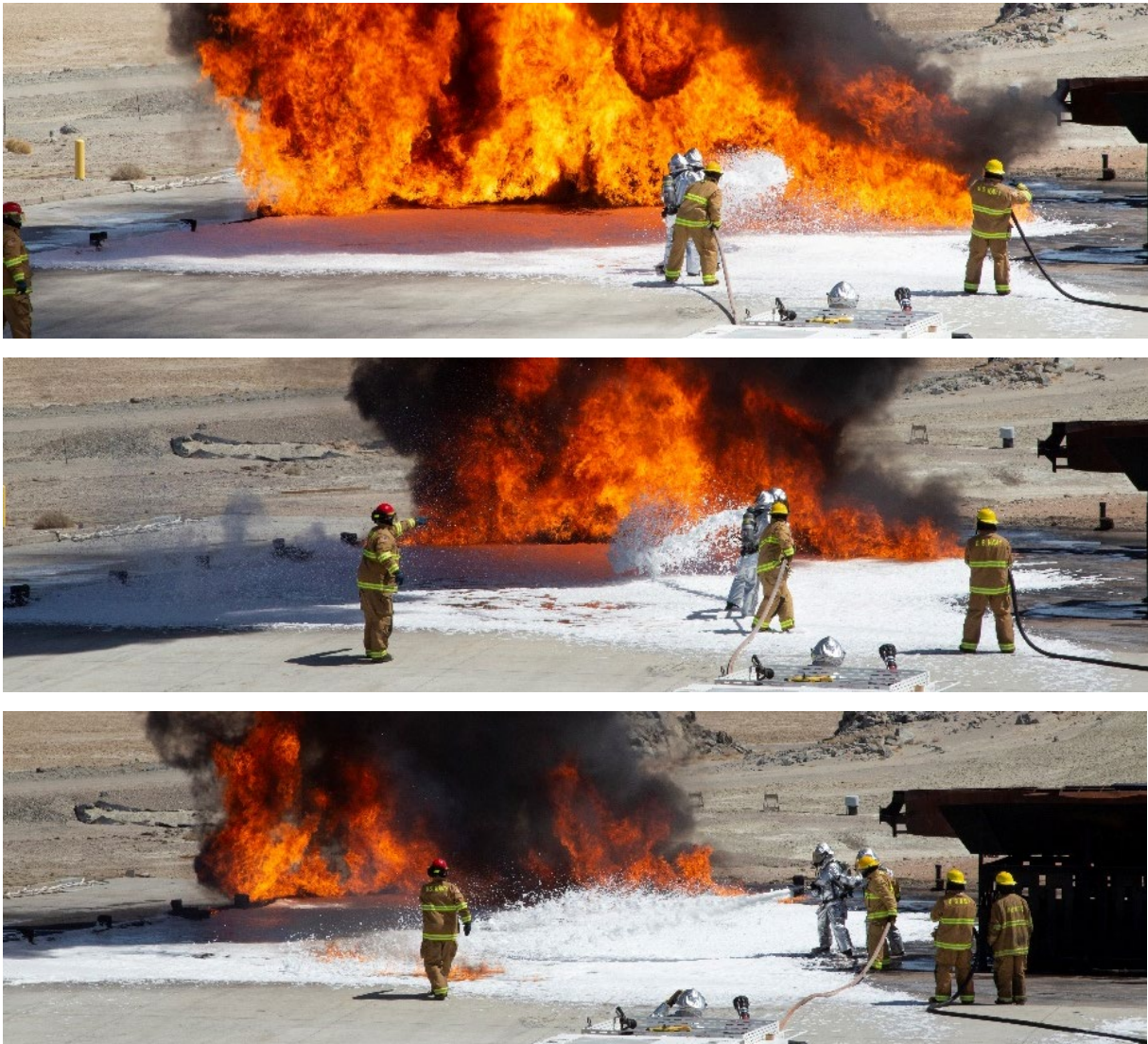
Fig. 4.2-2 – Openings in F3 Aspirated Foam Blanket
