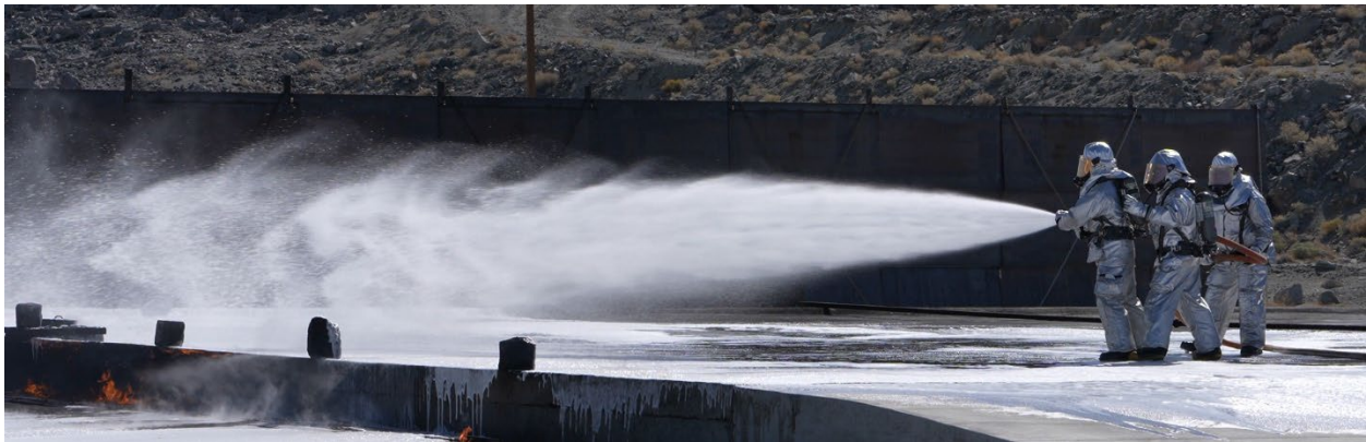
Fig. 4.4-3 – Slightly Wider Spray Pattern Used for Close-in Application
