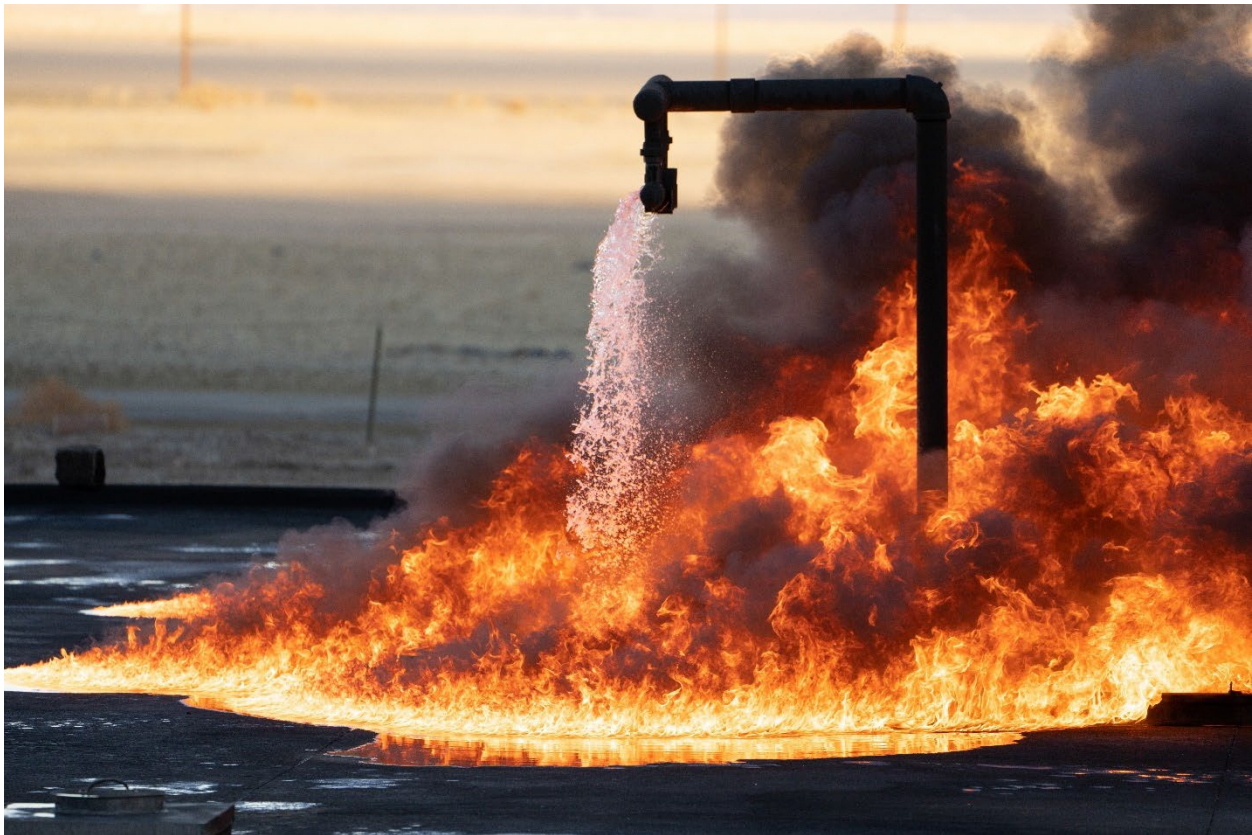
Fig. 4.6-1 – Flowing/Running Fuel Fire Scenario
