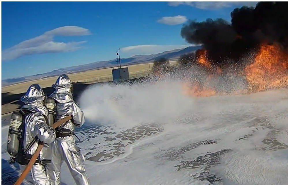
Fig. 4.5-3 – Rapid Foam Breakdown Shortly After Application
