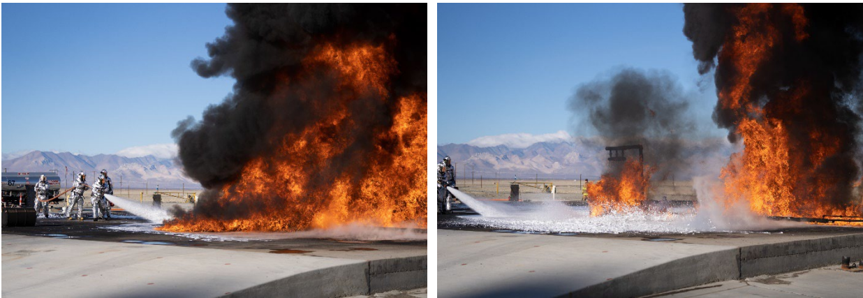
Fig. 4.6-2 – Roll-on Foam Application Pushing Toward the Base of the Falling Fuel
