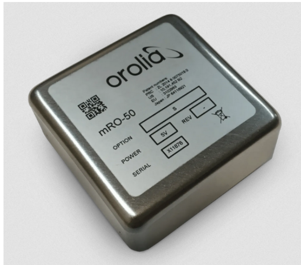
Figure 6. Orolia Miniaturized Rb Oscillator [15]
