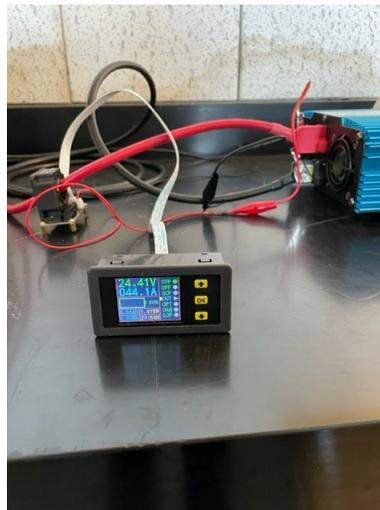
Figure 4.10. Bidirectional volt/amp meter
