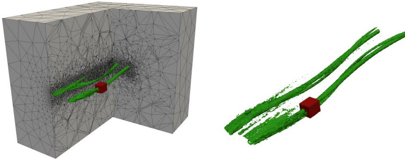
Figure: Simulation output for counter-rotating vortices from high order simulation. Note the variation of element sizes from the region of interest to boundaries. The L-SIAC filter needs to be scaled dynamically to obtain meaningful results.
