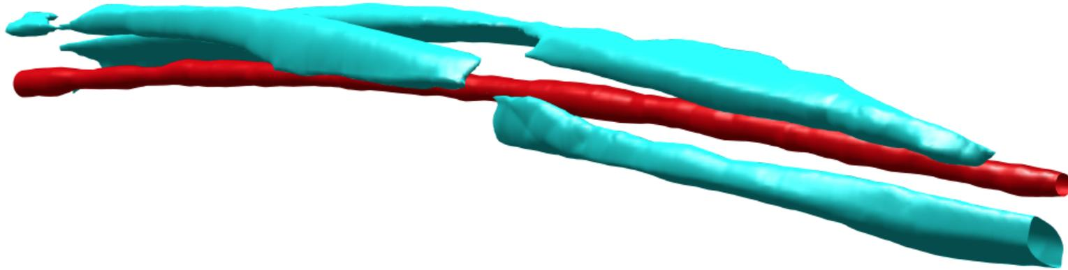
Figure 13: The red iso-surface is the primary vortex with  $\Lambda^{-2}$  value of 8000, and cyan iso-surface represents the secondary counter rotating vortex with  $\Lambda^{-2}$  value of -750. For this visualization, we have used the adaptive scaling of L-SIAC filter combined with efficient implantation of the L-SIAC filter.
