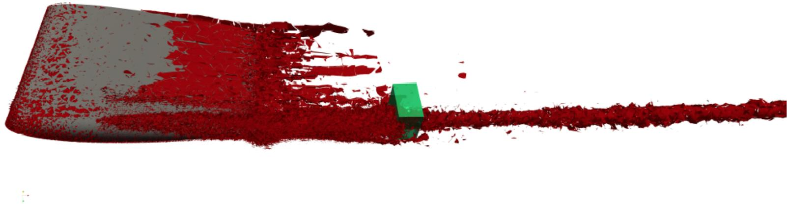
Figure 2: Large-Eddy Simulation (LES) for the formation and evolution of a wingtip vortex. The wing is a 3D extrusion of a NACA 0012 airfoil section with a rounded wing tip and a blunt trailing edge. Angle of attack  $=12$ . The green cube shown in the vortex, downstream from the tip, indicates the selected region that will be used to more closely examine the vorticity field.
