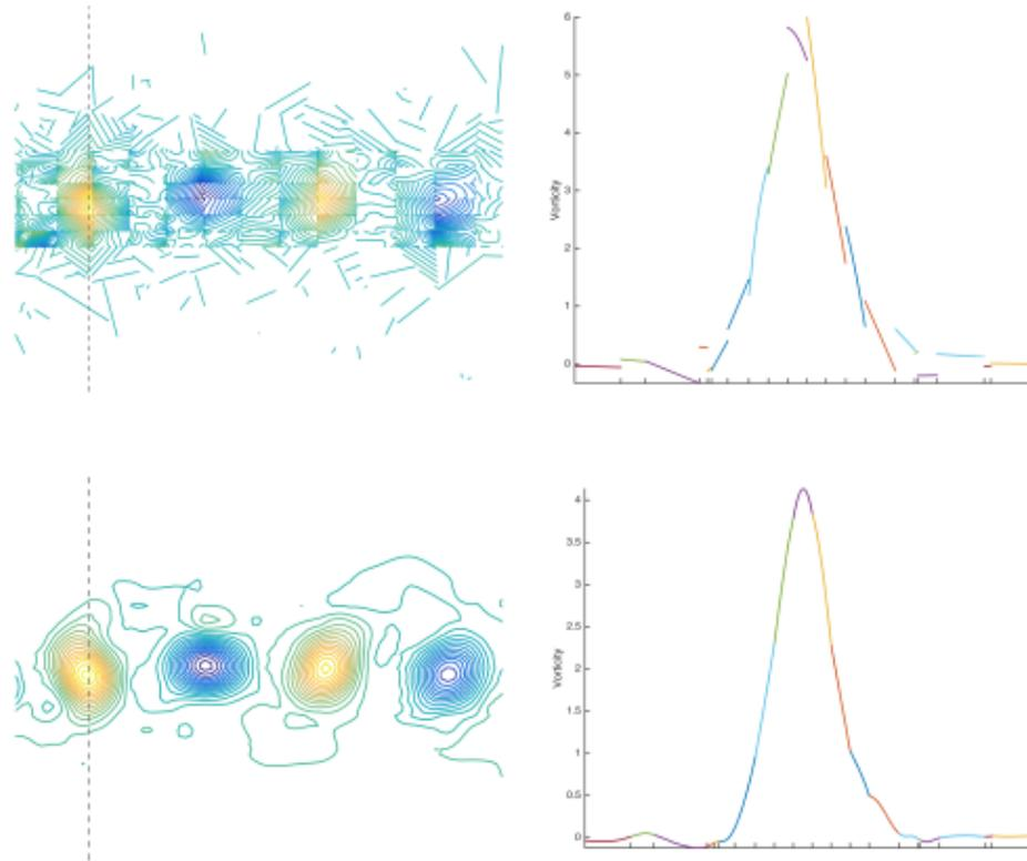
Figure 1: Images from Cylinder Flow. Comparison between calculating vorticity using dG data vs L-SIAC. The first row of images are calculated using raw dG data at fine grid resolution. Second Row of images are vorticity calculated L-SIAC.
