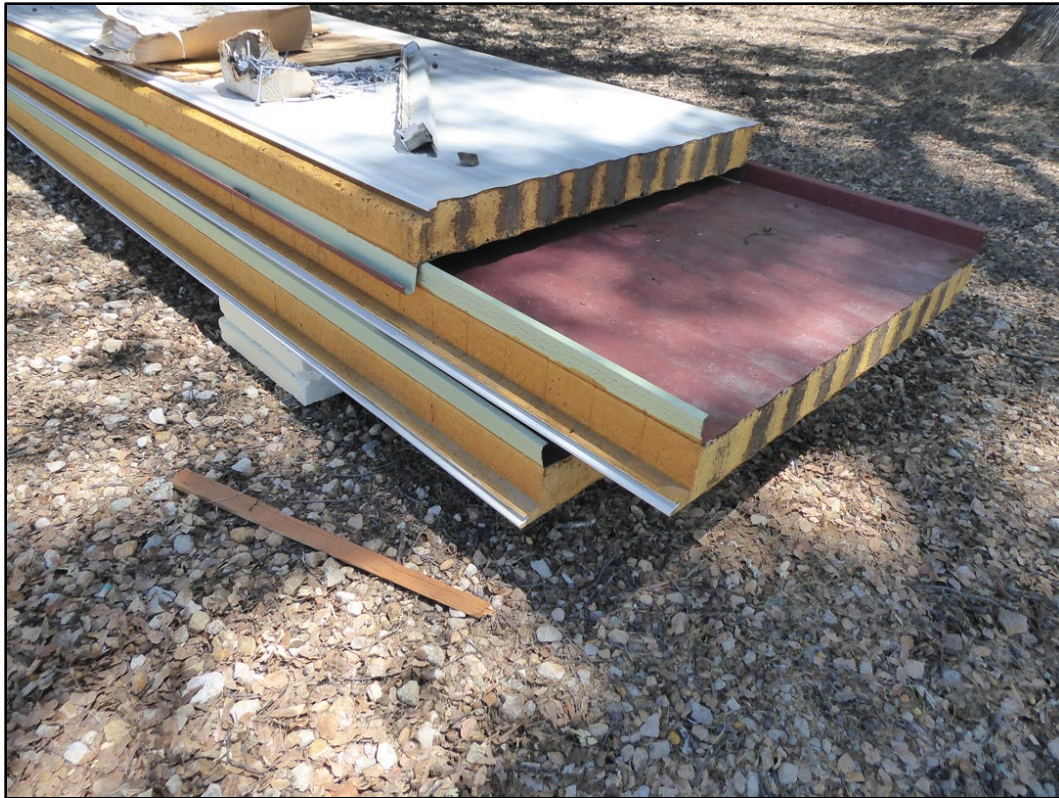
Figure 105. Kingspan insulated panels used on the exterior of Building 291. (ERDC-CERL, 2021. Public domain.)
