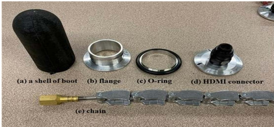
Figure 8. Components used for assembling sensor housing
