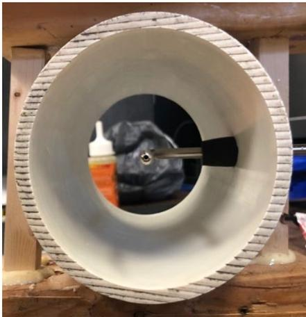
**Fig. 3.** The Pitot tube incorporated into the tube to determine the volumetric flow rate.
