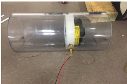
Figure 3. The installation of the two-stage axial fan into the butyrate tube.
