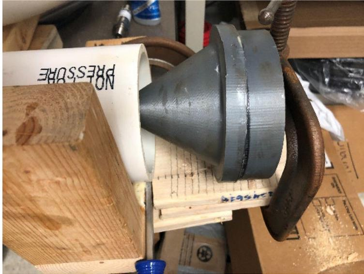
*Figure 51(b). Shows how the flow was regulated and the mounting structure to maintain the flow axisymmetric.*
