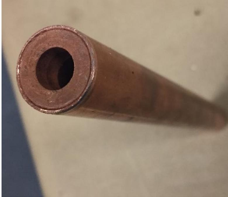
*Figure 115. Pipe 3, un-sintered copper powder wick heat pipe*
