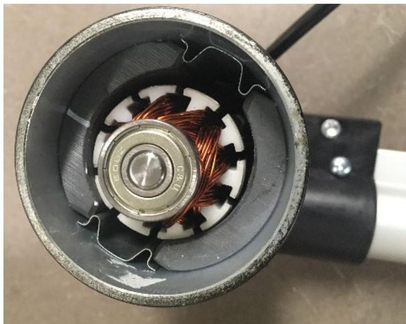
127(b). Inside view of motor shows copper windings embedded in rotor core and separated by a clearance. The stator is a permanent magnet.
