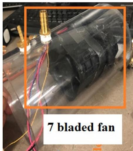
*Figure 154. The Delta dual fan system and its incorporation into the clear tube, Fan 2*
