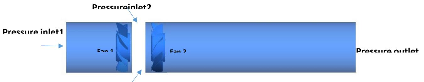
Fig. 19 Computational domain and boundary condition for the open wall case
