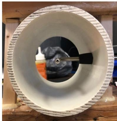
*Figure 149. The Pitot tube incorporated into the tube to determine the volumetric flow*
