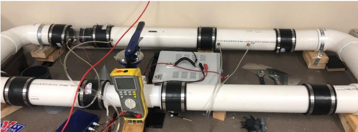
**Figure 51. The experimental loop that incorporates the butterfly valve as the flow restriction device and in the test loop laying flat on the table (experimental setup 1).**
