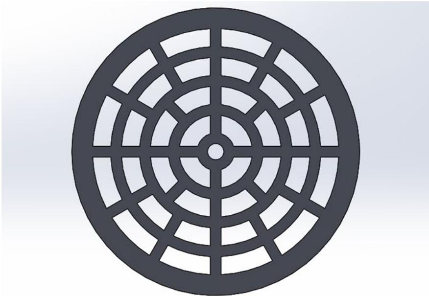
*Figure 25. Flow straightener used in the simulation*
