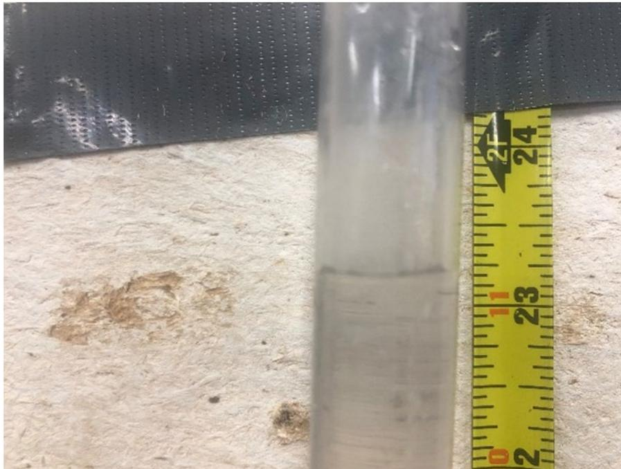
***Figure 40. Water Level was Determined by Carefully Reading the Level at the Meniscus***
