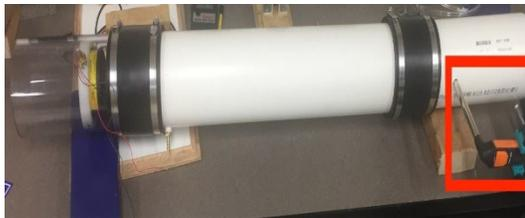
Figure 10. Measurement of the air velocity using the probe (red box).
