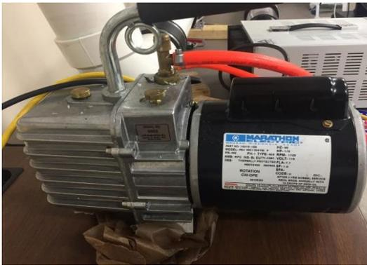
Figure 5. The vacuum pump used in the loop.
