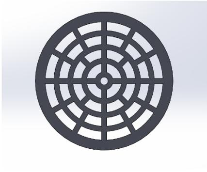
Figure 8. Flow straightener used in the simulation.
