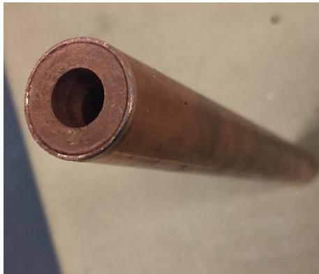
Fig. 2. Pipe 3, un-sintered copper powder wick heat pipe
