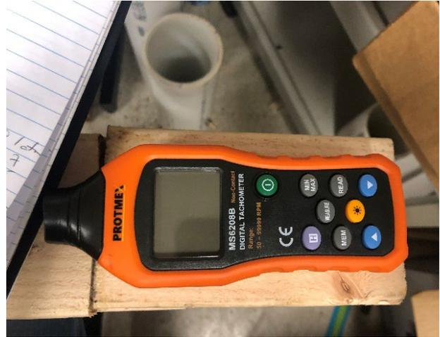
**Fig. 5b.** The Protmex non-contact tachometer used to verify the fan's rotational speed.
