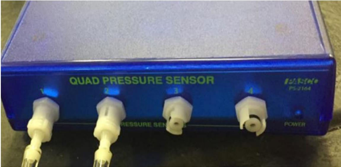
**Figure 8. The PASCO Quad Pressure Sensor**
