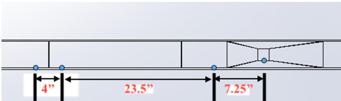
*Figure 19. Pressure Taps in the Simulation are Placed in Identical Positions as the Experimental Taps*
