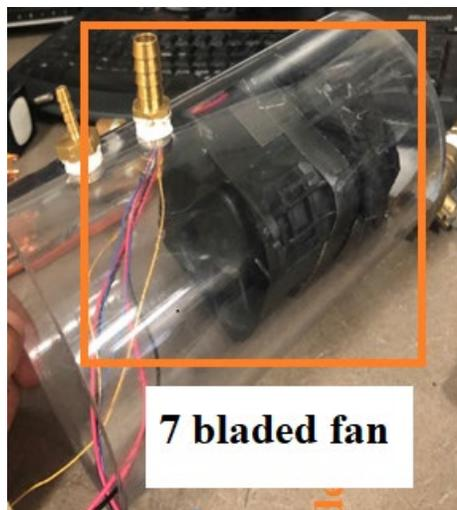
**Fig. 8.** The Delta dual fan system and its incorporation into the clear tube, Fan 2.
