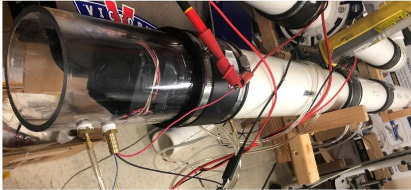
**Figure 54.** *The experimental setup used to develop the fan performance curves when using the cone as the flow restricting device (experimental setup 2).*
