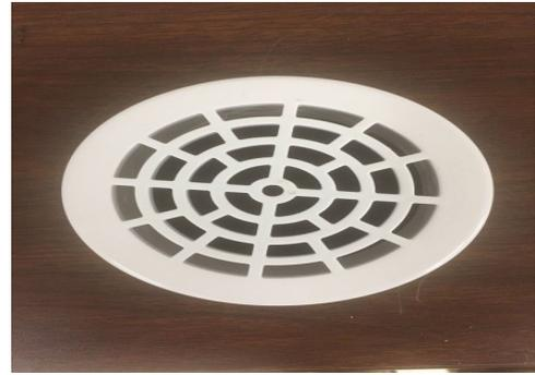
Figure 11. The flow straightener used.
