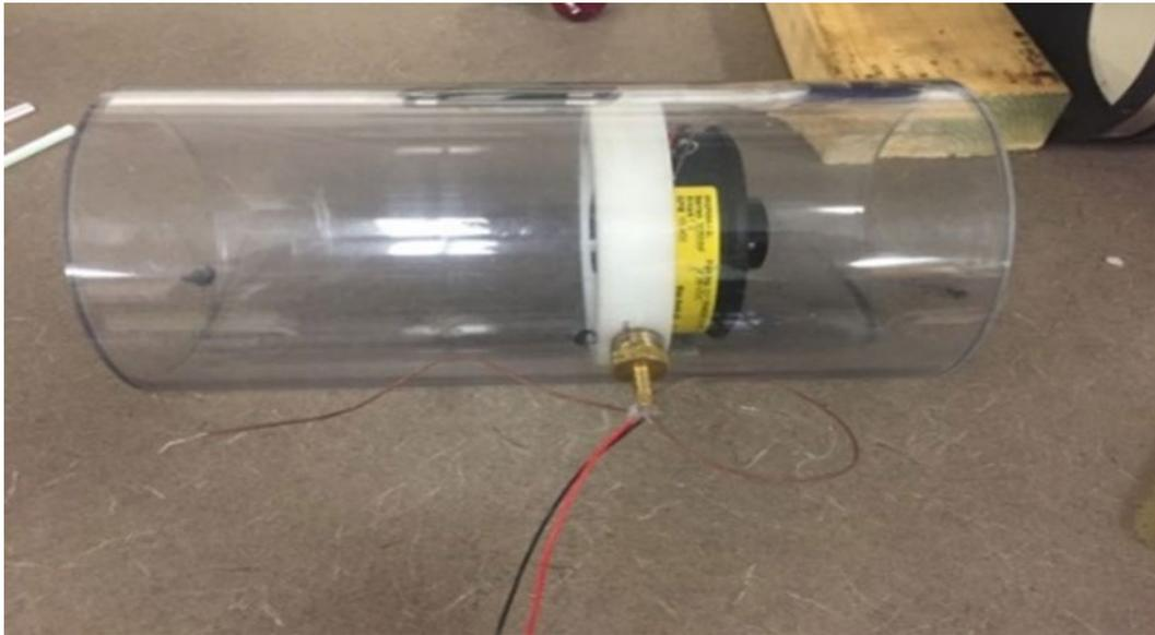
**Figure 20. The Installation of the Two-stage Axial Fan into the Butyrate Tube**
