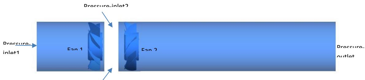
Fig. (8) Boundary conditions for the opened wall case
