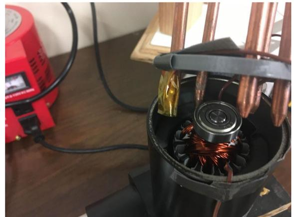
Figure 3: inside view of motor showing heat pipe evaporators
