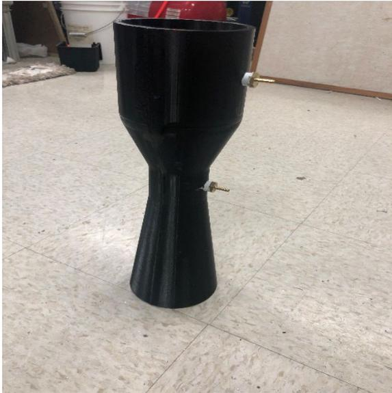
**Fig. 2.** The 3D printed ABS Venturi,  $\beta = 0.51$ .
