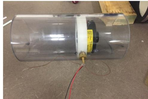
Figure 2. The fan and butyrate clear tube assembly.
