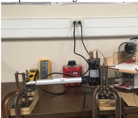
c. PA 03 EMA with 5 heat pipes extending through the cover
