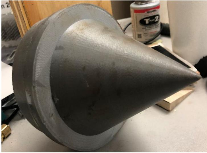
*Figure 52. 3D printed cone used for restricting the flow to obtain the fan*
