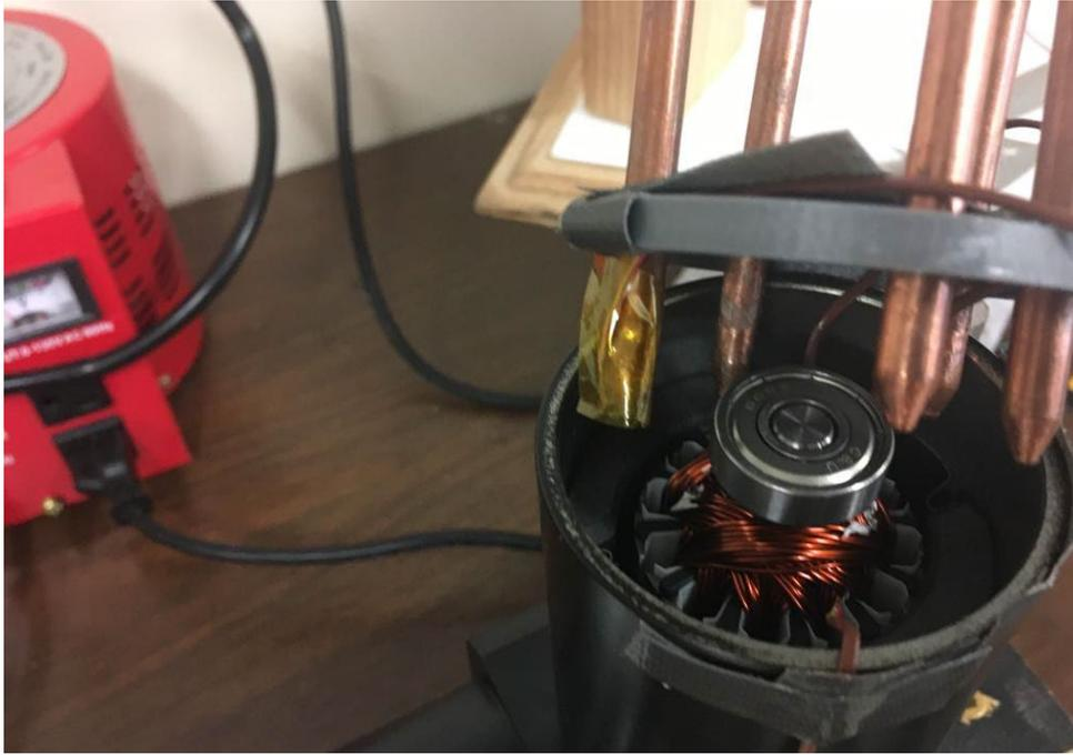
*Figure 130. Inside view of motor showing heat pipe evaporators*
