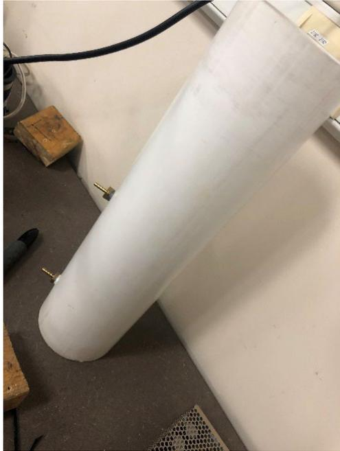
**Figure 61 (b). Nylon machined venturi,  $\beta = 0.46$**
