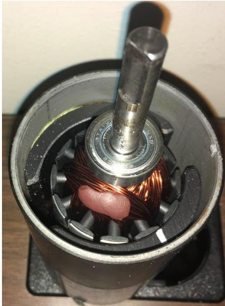
*85(c) Rotor and stator assembly.*
