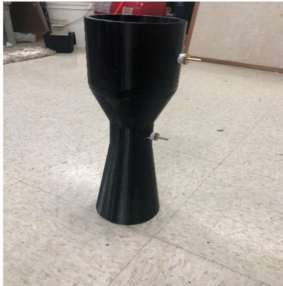
*Figure 148. The 3D printed ABS Venturi,  $\beta = 0.51$ .*
