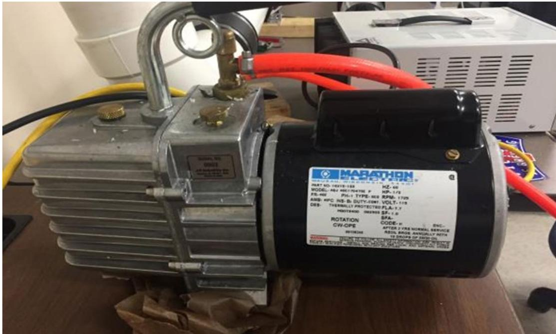
**Figure 5. The Vacuum Pump Used in the Loop**
