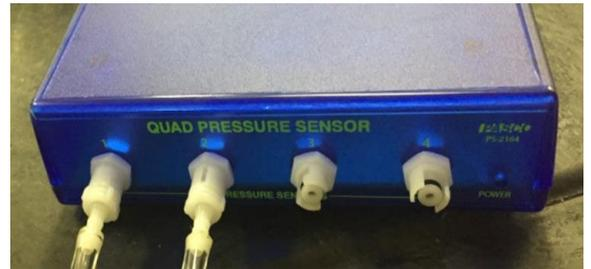
Figure 8. The PASCO Quad Pressure Sensor.
