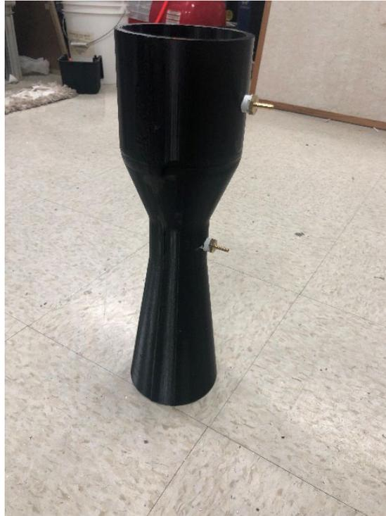
*Figure 62. (a). 3D printed PLA venturi,  $\beta = 0.51$ .*
