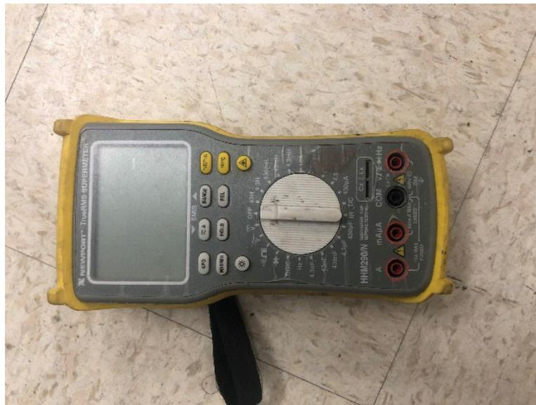
**Figure 47. (b)** Newport Super meter multi-meter used in monitoring the voltage output of the pressure
