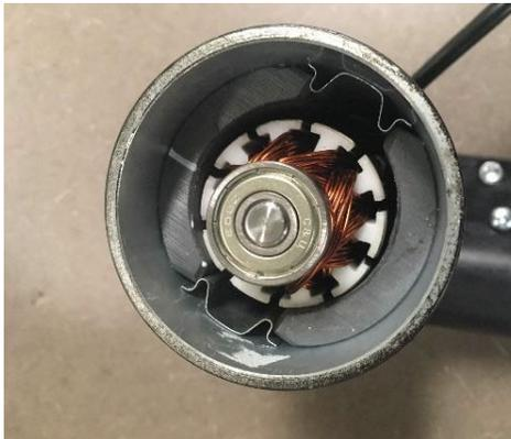
b. Inside view of motor shows copper windings embedded in rotor core and separated by a clearance. Stator is a permanent magnet
