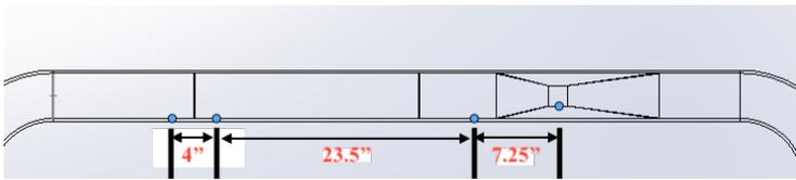
Figure 2. Pressure taps in the simulation are placed in identical positions as the experimental taps.
