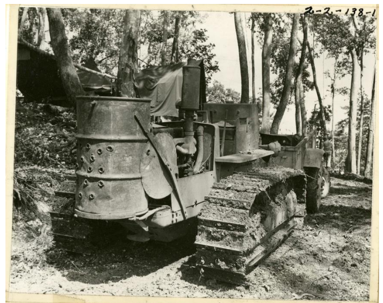
Radiator repair done by Seabees from the 73rd Naval Construction Battalion with a 55-gallon drum, Munda, Solomon Island
