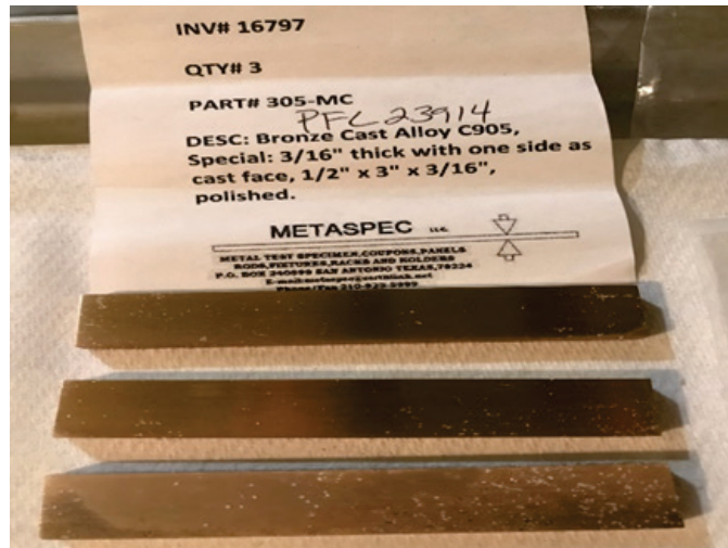
Figure 6. Post-test condition of 305-MC test specimens.
