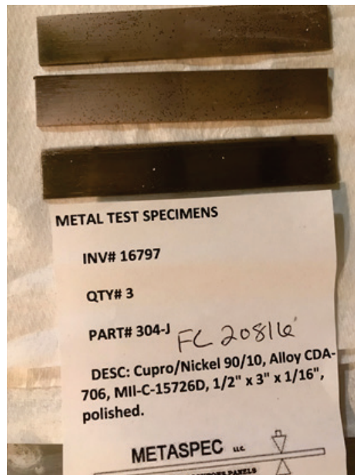
Figure 7. Post-test condition of 304-J test specimens.
