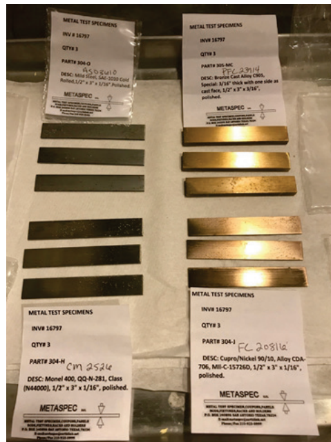
Figure 3. Post-test condition of the four test specimens.
