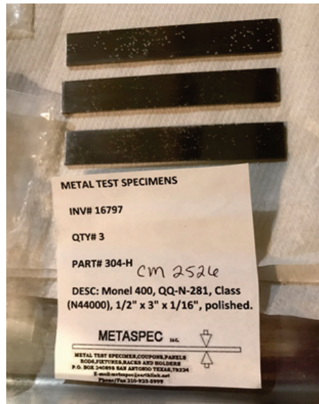
Figure 4. Post-test condition of 304-H test specimens.
