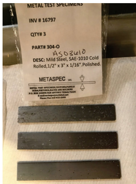
Figure 5. Post-test condition of 304-O test specimens.
