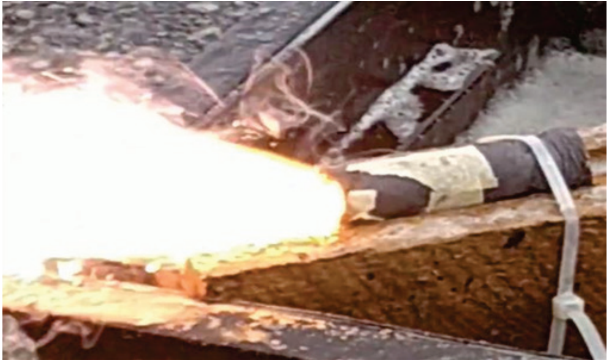
Figure 12. Pyrotechnic underwater flare, fully ignited.
