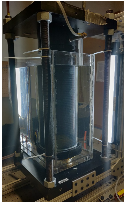
Figure 8. Custom designed Taylor Couette Cell
