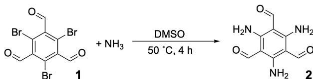
Fig. 1 Synthesis of 2,4,6-triaminobenzene-1,3,5-tricarboxylaldehyde, 2 , from Rubin's aldehyde, 1 , using anhydrous ammonia in dimethyl sulfoxide (DMSO)
