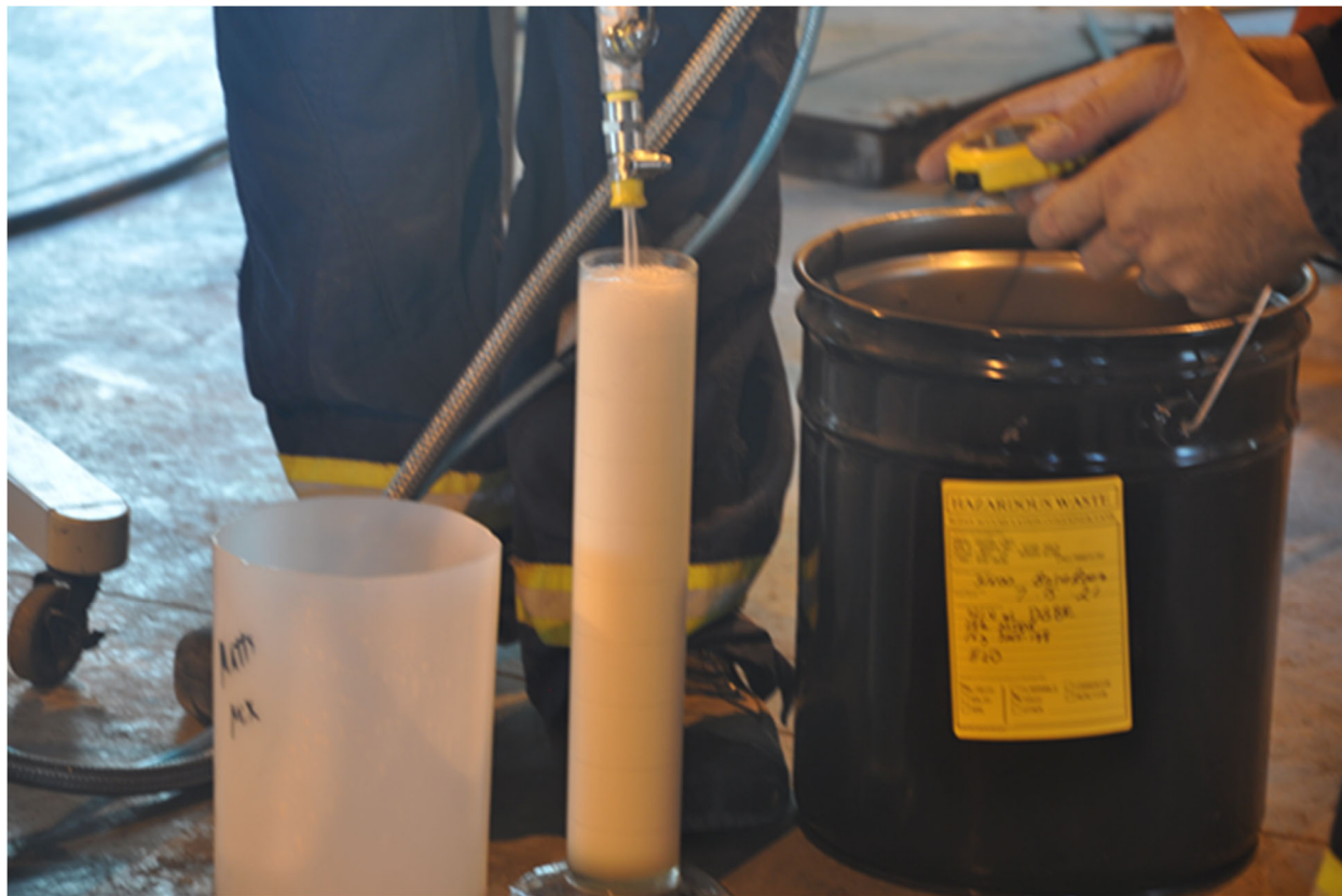
Figure 94 Foam expansion test of surfactant 2062-145/225DK/DGBE with 1 L graduate cylinder.
