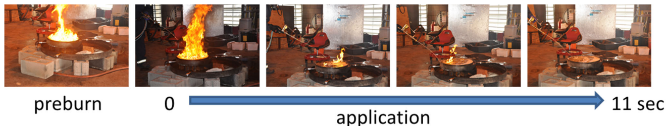
Figure 98 Fire extinguishment experiment with 2062–139/225DK/DGBE in water. The mixture was able to extinguish the 20 square inch F24 pool fire in an average of 11 seconds.
