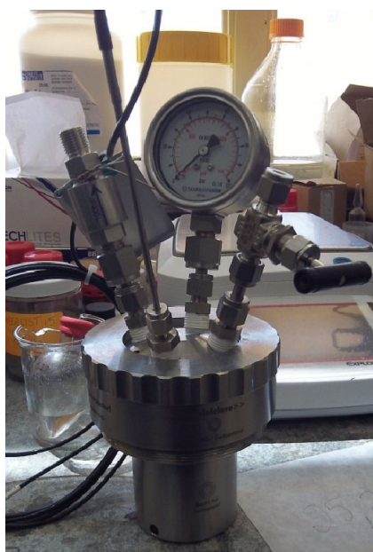
Figure 22 Stainless steel Buchiglas miniclave, a high pressure autoclave used in the amination reaction.
