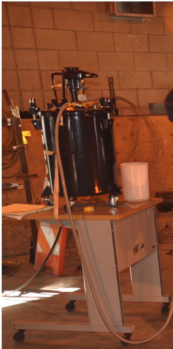
Figure 88 An inexpensive, air regulated generic five gallon pressure paint pot was adapted and used to generate and apply surfactant solutions in pool fire testing.
