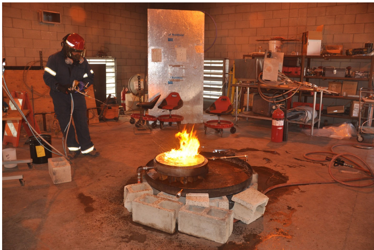
Figure 10 Photograph during extinguishment test with the 2062–145/225DK/DGBE mixture showing the CAFS nozzle in action to put out the 20 square inch F24 pool fire.
