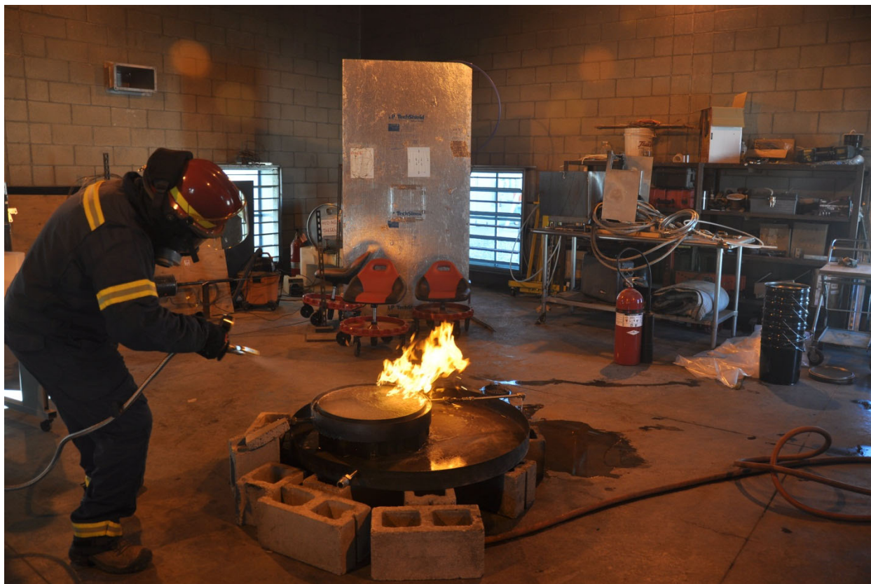
Figure 95 Photograph during ES1#3 test with flowrate doubled, showing the fire fighter had to employ multiple tactics with the NF04 nozzle to put the fire out. One can see the very fine spray created from the simple fan DETE NF04 nozzle which did not create very much foam from the nozzle.
