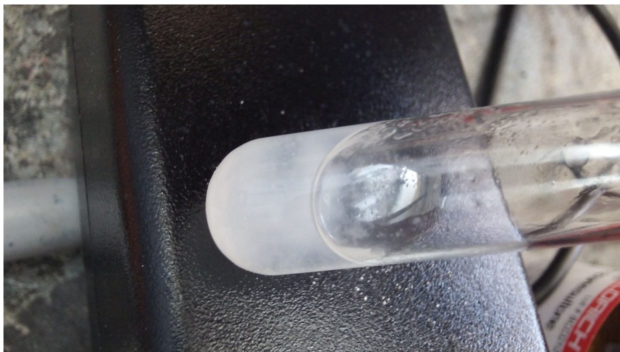
Figure 48 The monogluconamide 2062-172 would not dissolve in water but remained a suspension for one month.
