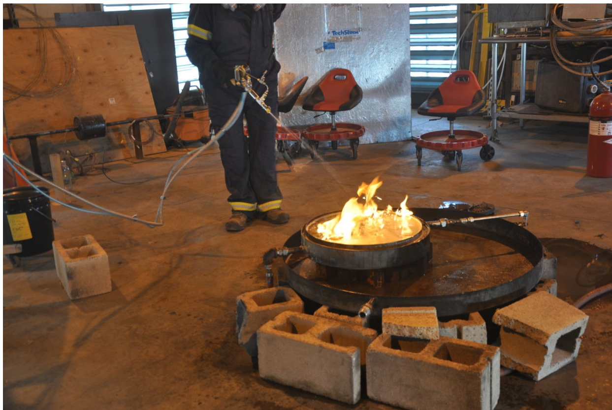
Figure 96 Photograph during ES1#6 test showing the CAFS nozzle in action, the fire fighter could stand in one spot and put out the fire with the better quality foam created by the CAFS nozzle.
