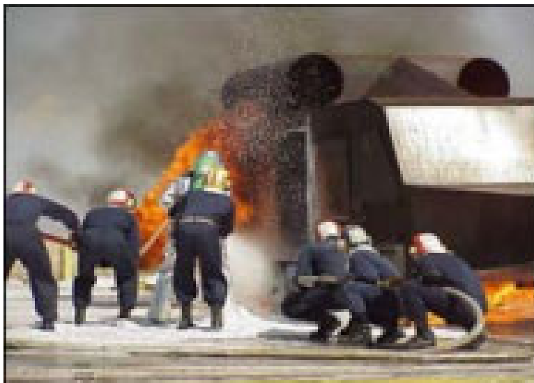
Figure 11 Navy fire crew extinguishing hydrocarbon pool fire at a test facility with aqueous film forming foam (AFFF).
