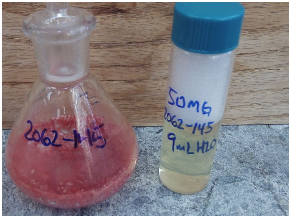
Figure 49 The bisgluconamide 2062-145 would slowly and completely dissolve in water and gave an apparent surfactant solution that foamed when shaken vigorously.
