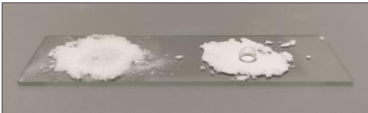
Figure 7. Comparison of water droplet behavior over as-purchased HGMs (left) and 3-Trimethoxysilyl propyl Chloride then HMDSO-reacted HGMs (right)
