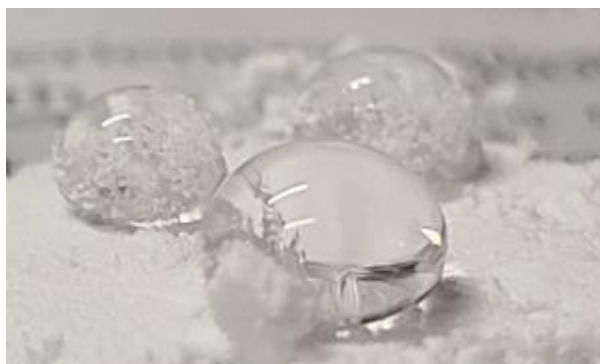
Figure 28. Behavior of hydrolyzed MTMS coated A20 microspheres.
