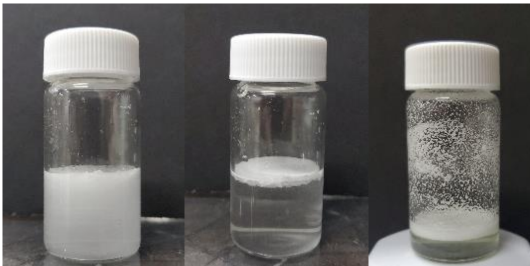
Figure 14. PVB treated microspheres in water immediately after being shaken (left image), PVB treated microspheres in water 5 minutes after being shaken (middle image), and PVB treated microspheres in gasoline immediately after being shaken
