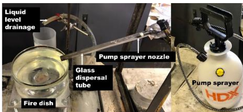
Figure 23. Photographs of new HGM foam sprayer setup
