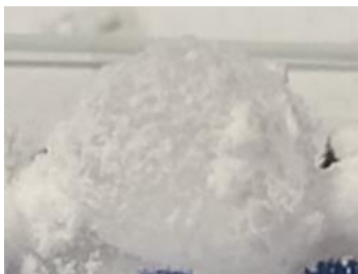
Figure 29. Behavior of hydrolyzed MTMS coated A20 microspheres.
