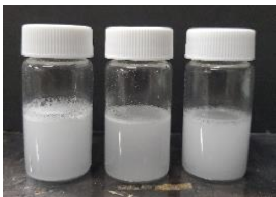
Figure 10. From right to left, PVA treated microspheres 1, 2, and 3 in water immediately after being shaken
