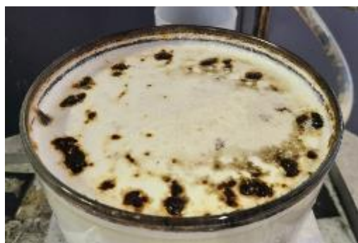
Figure 33. Foam layer of 4% K37 with siloxane surfactant and polysaccharide after unsuccessful fire testing.
