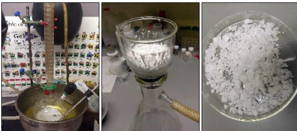
Figure 6. HGMs being reacted with HMDSO (left), being dried using vacuum filtration (center), and final product obtained (right)
