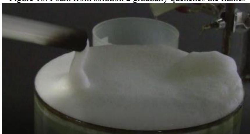
Figure 19. Foam from solution 2 successfully quenches the flames
