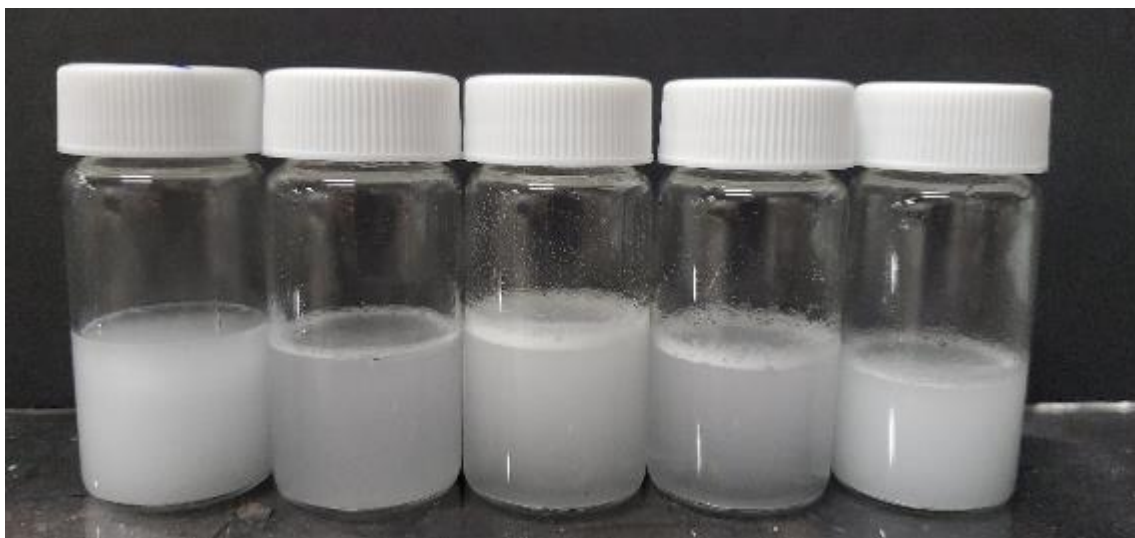
Figure 12. From right to left, PEG treated microspheres 1, 2, 3, 4 and 5 in water immediately after being shaken
