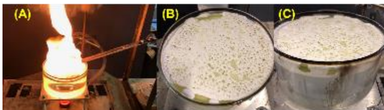
Figure 24. Photographs of (A) fire testing, (B) and (C) uncoated-HGMS on top of gasoline after fire testing
