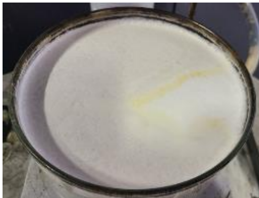
Figure 32. Foam layer of K37 and commercial sodium lauryl sulfate surfactant solution with streaks of gasoline after unsuccessful fire testing.
