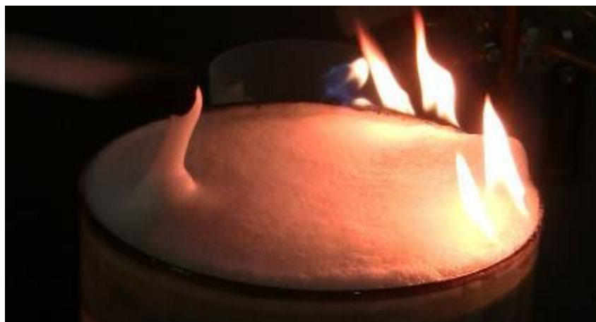
Figure 18. Foam from solution 2 gradually quenches the flames
