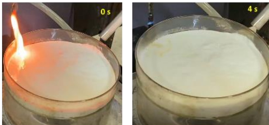
Figure 36. Self-quenching action of glass microspheres of gasoline pool fire
