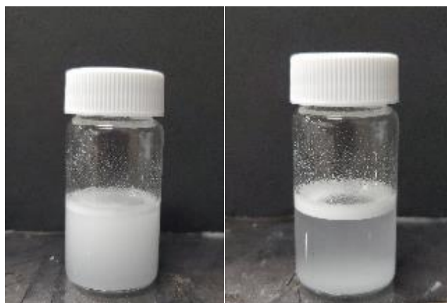
Figure 16. CMC treated microspheres in water immediately after being shaken (left image), CMC treated microspheres in water 5 minutes after being shaken (right image)
