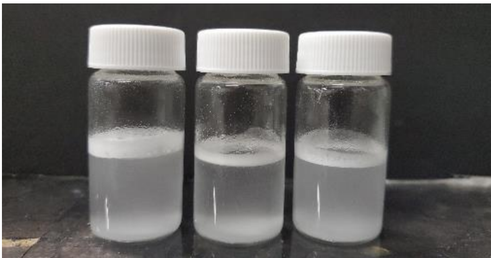
Figure 11. From right to left, PVA treated microspheres 1, 2, and 3 in water 5 minutes after being shaken
