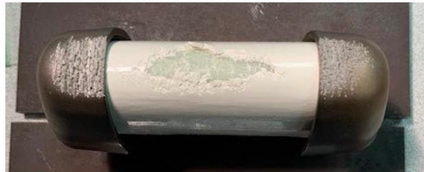
Figure 4: Specimen ID 1-2 after Rain Exposure at 440 MPH
