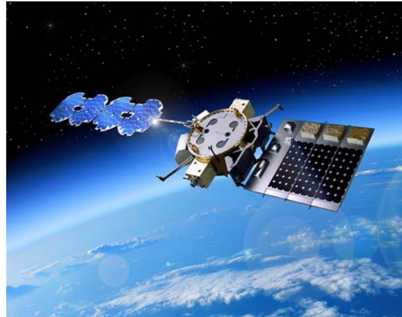
Figure 43. AFRL’s ARACHNE will serve as the first free-flying flight experiment needed to mature critical technologies deemed essential to building an operational solar power transmission system. (Credit: AFRL) 289
