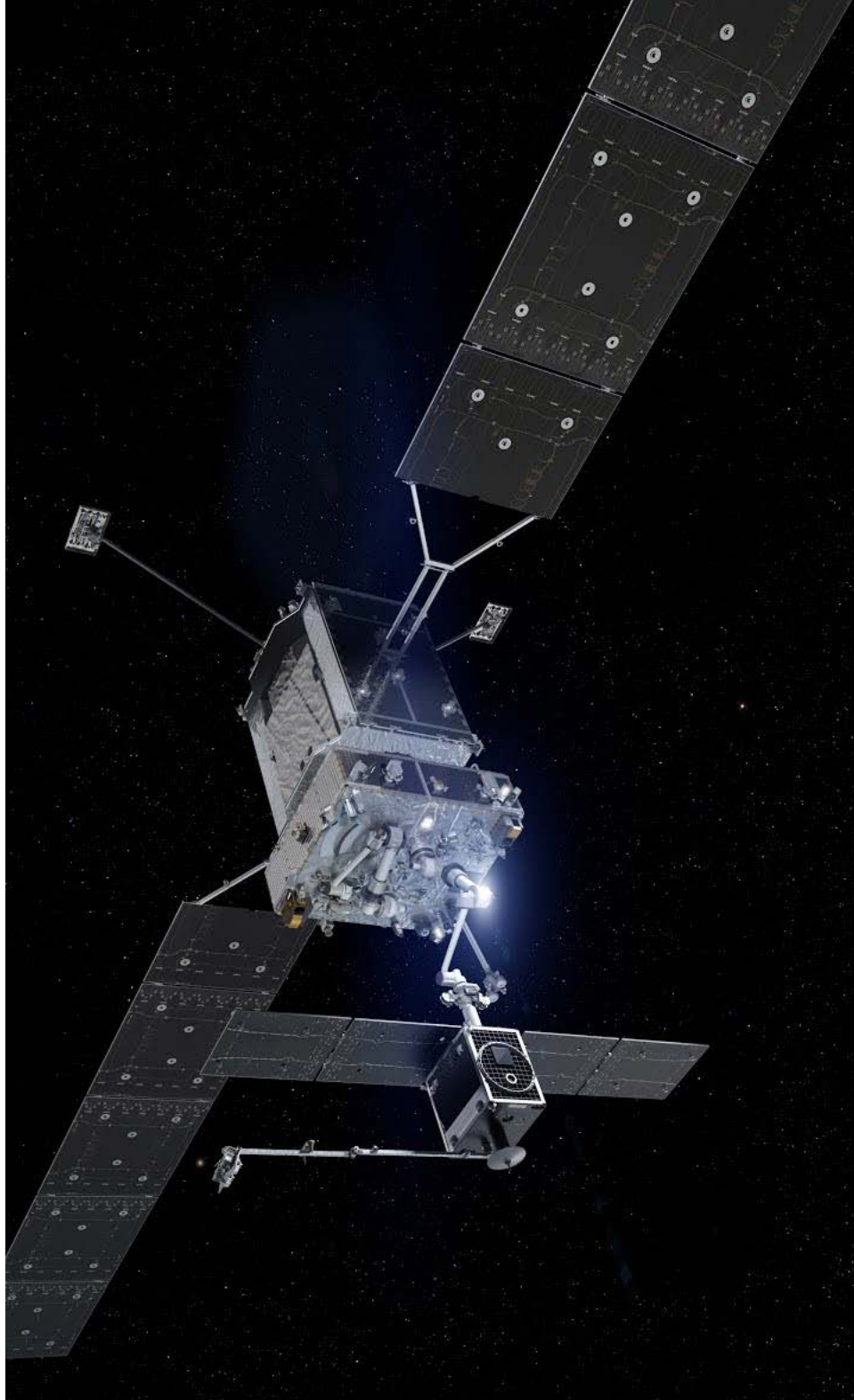
Figure 35. Space Logistics' Mission Robotic Vehicle (MRV) servicing a client satellite in geostationary orbit. (Credit: Northrop Grumman)
