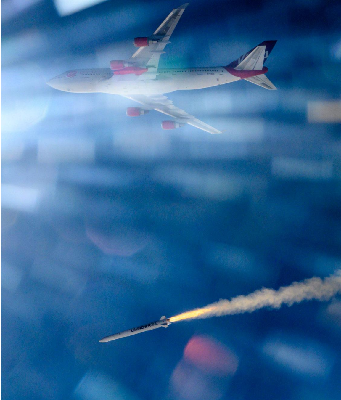
Figure 20. LauncherOne released from Virgin Orbit's modified Boeing 747 aircraft named 'Cosmic Girl' demonstrating the flexibility of airborne launch. (Credit: Virgin Orbit)
