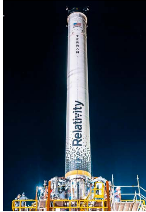
Figure 22. First stage of Relativity’s 3-D printed Terran 1 rocket at launch site. (Credit: Relativity)
