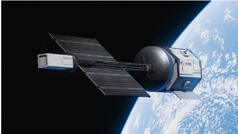
Figure 42. Artist rendering of the Shadow Runner spacecraft design utilizing ‘next-gen’ high power radioisotope source. (Credit: USNC-Tech)
