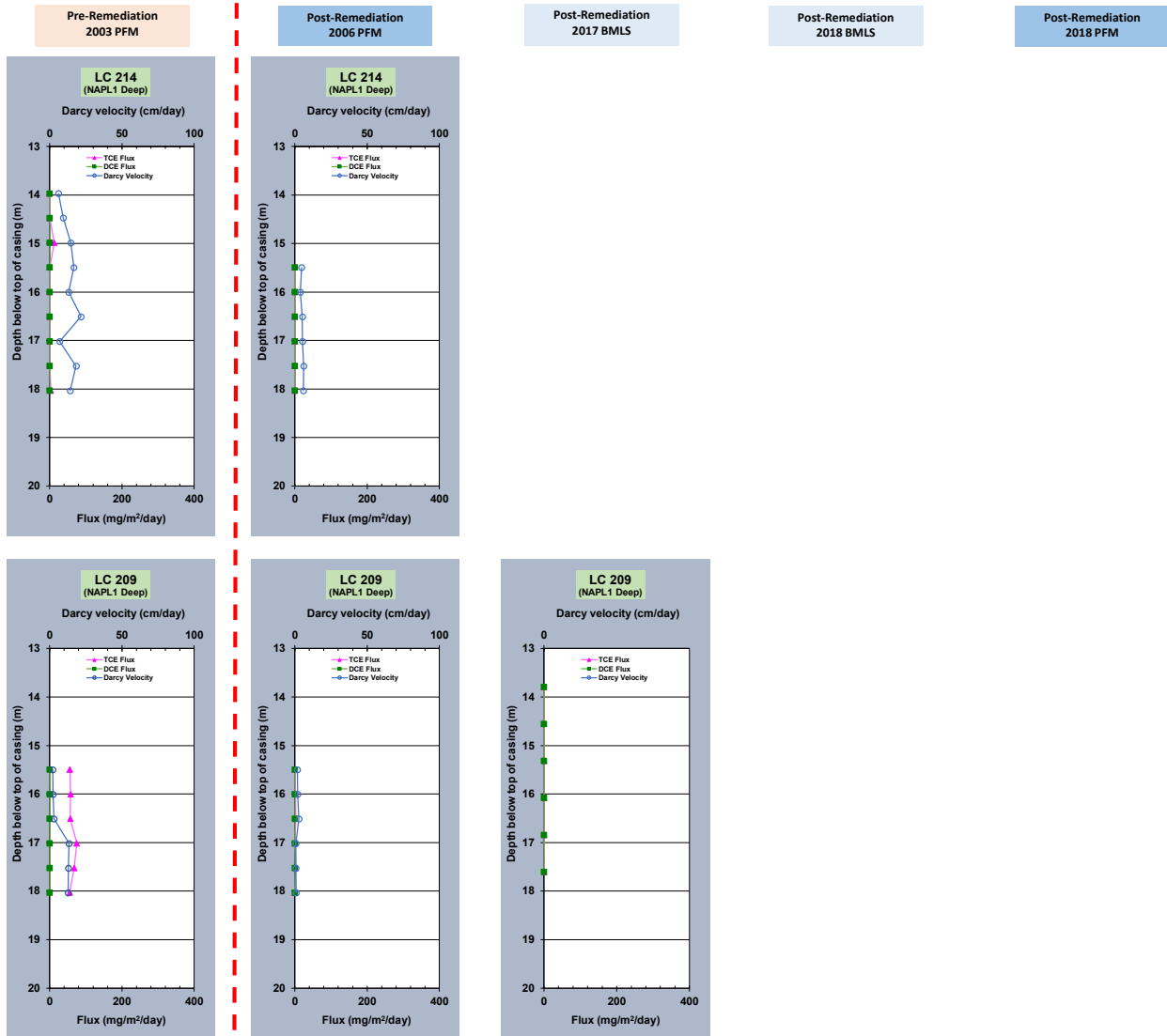
Figure 53. Comparison of Pre- and Post-remedial Fluxes Within the NAPL Area 1 Deep Well Flux Transect (Right Portion of Transect When Looking Down-gradient Through the Transect).
