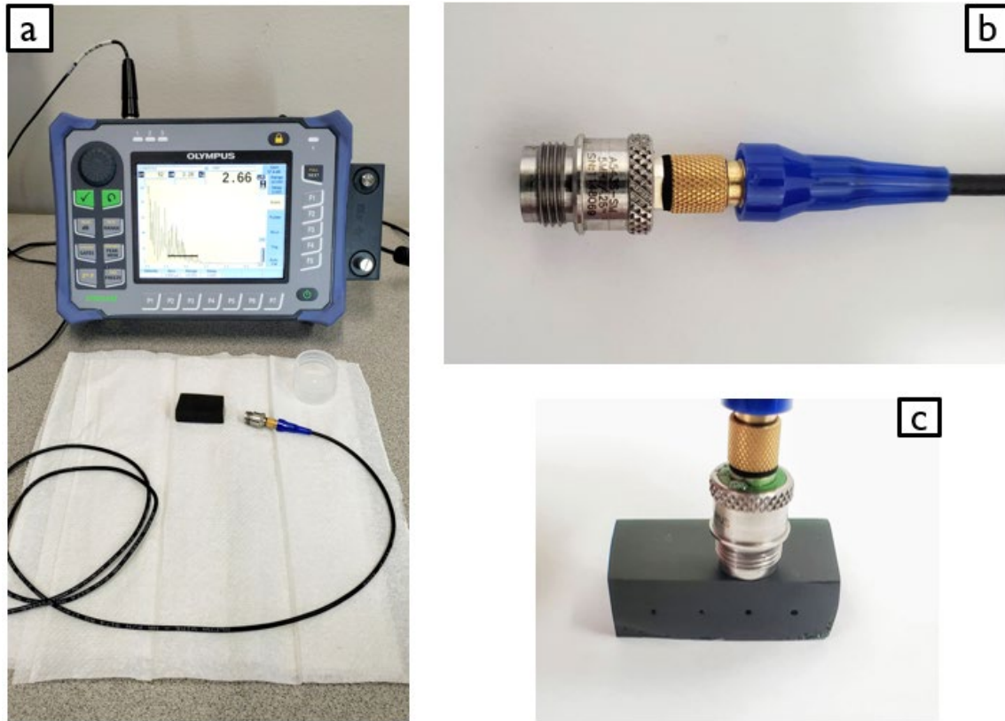
Figure 14. a) Olympus EPOCH 650 Ultrasonic Flaw detector, b) A543S-SM transducer and c) example transducer/sample configuration for flaw detection.
