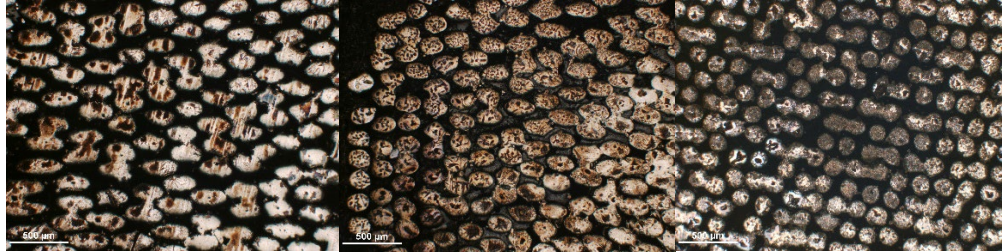
Figure 54. Variation in pillar geometry with CNT concentration (pure SS [a], 1 vol. % CNT [b] and 2 vol. % CNT [c])
