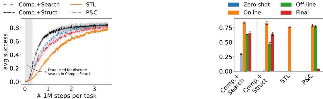
Figure 73: Avg. Success of STL and Lifelong Agents on 48 Compositional Robot Manipulation Tasks: (Left) During Training on Each Task and (Right) at Various Stages of Training
