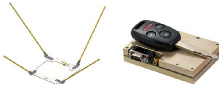
Figure 12. NanoCom ANT430 Antenna and TRX-U UHF Transceiver. Source: Left, [27]; Right, [28].
