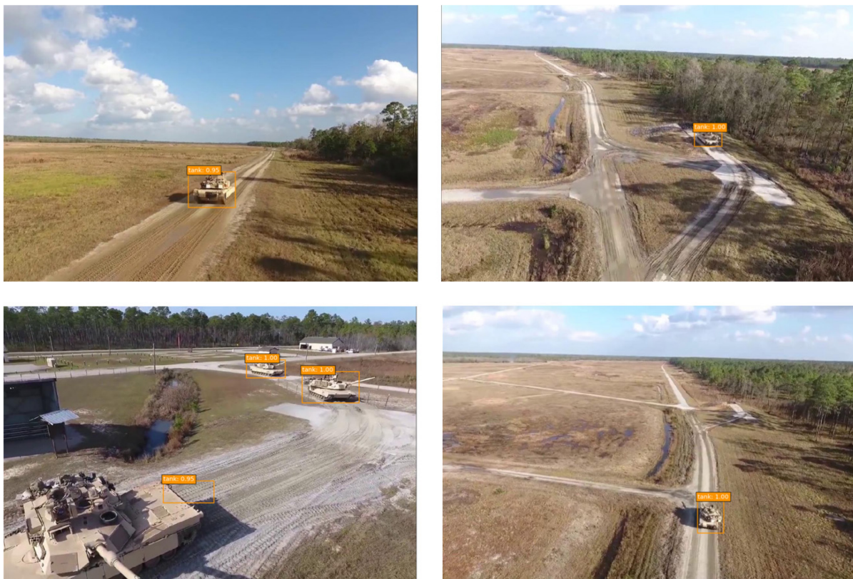
Figure 8: Some Examples of Detections of Our Tank Detector on Real Imagery. The viewpoints in these test images are close to the ones in the training data, see Figure 7.
