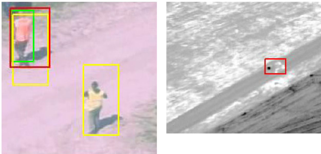
Figure 9: Three Complementary Detectors: ACF (Green), and Two MOD Variants (Yellow and Red).
