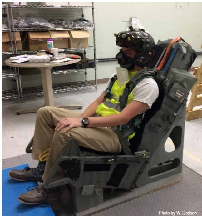
Figure 5-5: Subject Wearing the Foam Wedge to Support the Chin, to Offset the Forward Centre of Balance. Photos reprinted with permission from W. Dodson.
