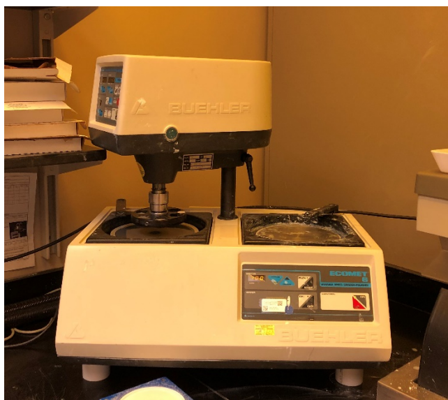
Picture 2: Buehler Automet 3 powerhead and Ecomet 6 Variable Speed Polisher
