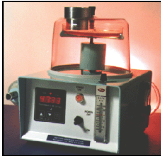
Figure 1. Mattson-Garvin model 220 slit-to-agar (STA) sampler.
