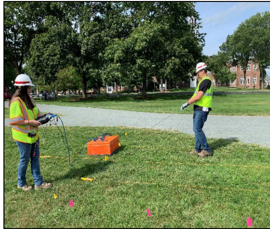
Figure 2. GPR data collection.
