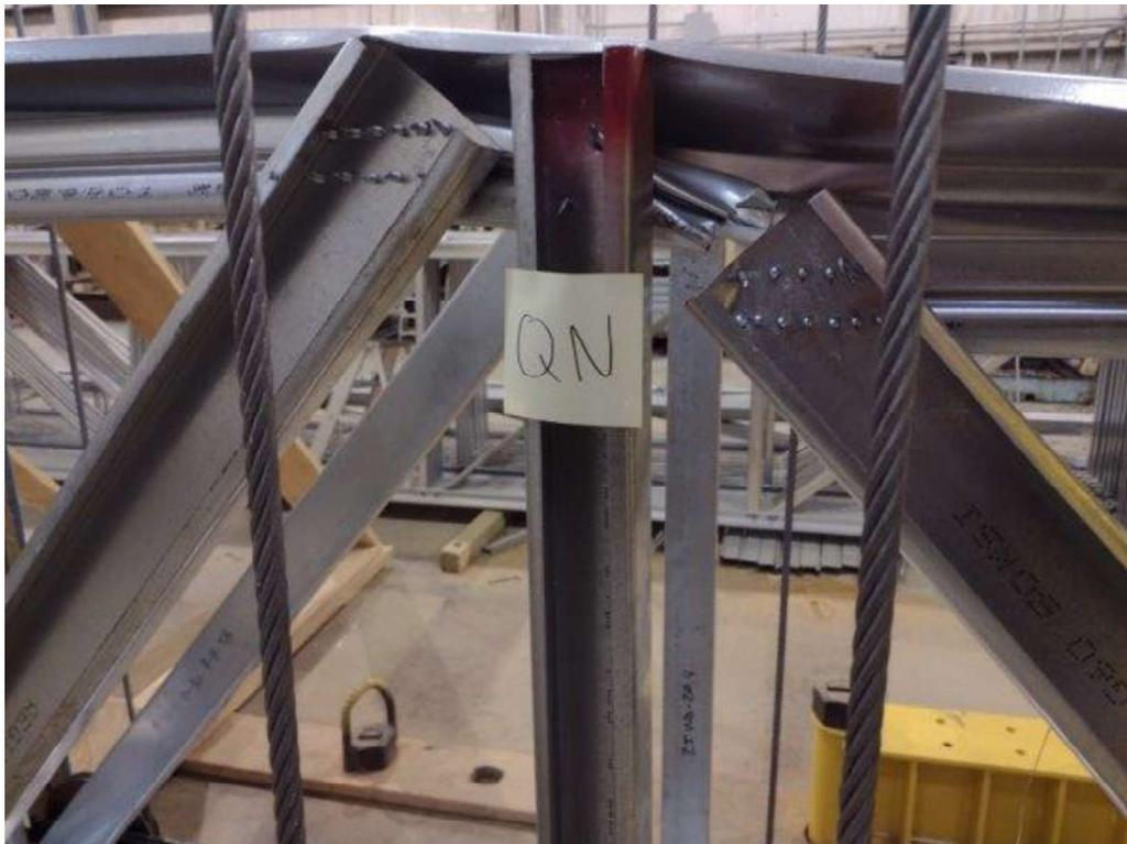
Figure 40: Beginning of Tension Chord Separation (AG48-D57)
