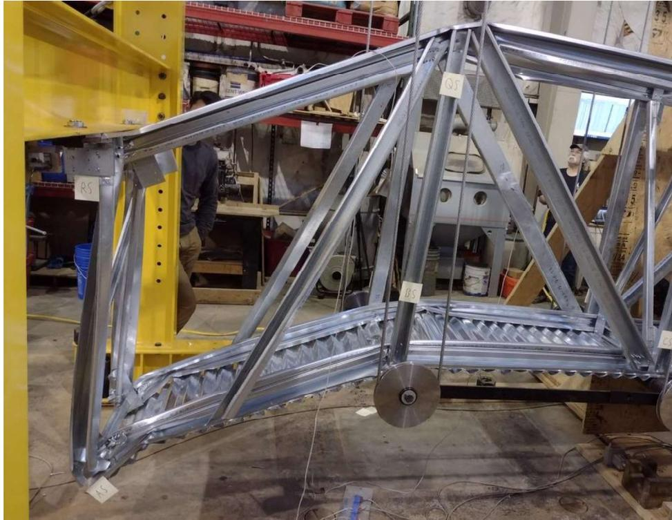
Figure 36: West Quarter of Specimen During Failure (AG48-D35)
