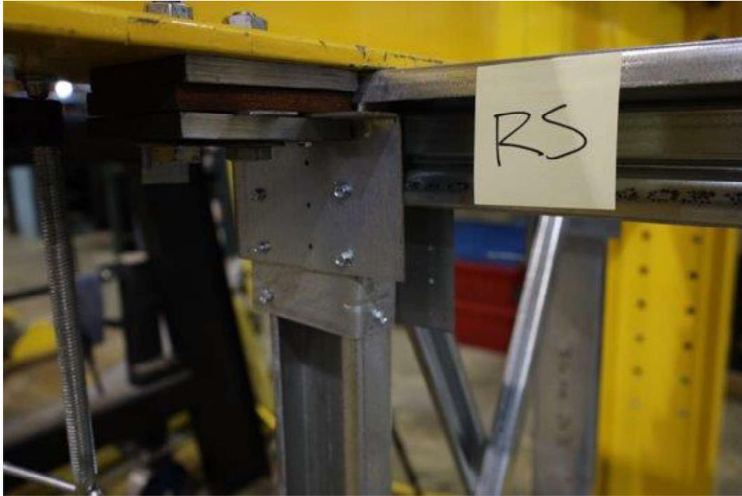
Figure 50: Specimen Setup - End Bearing
