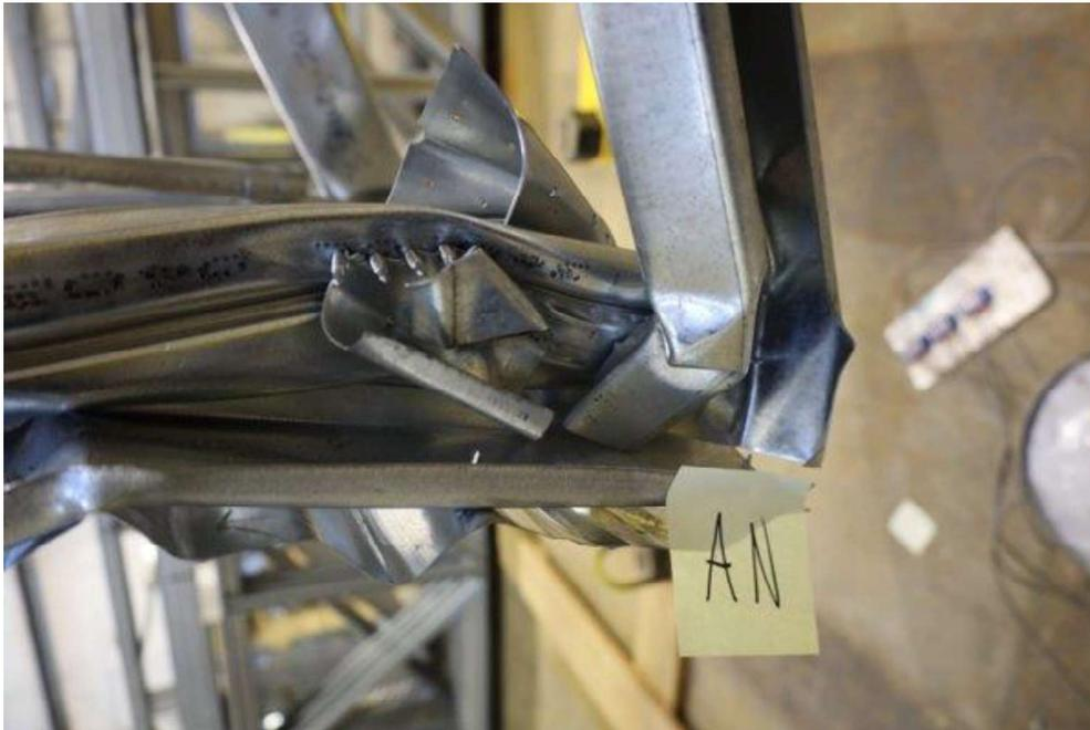
Figure 31: Rupture of Diagonal at Joint AN (AG48-D35)
