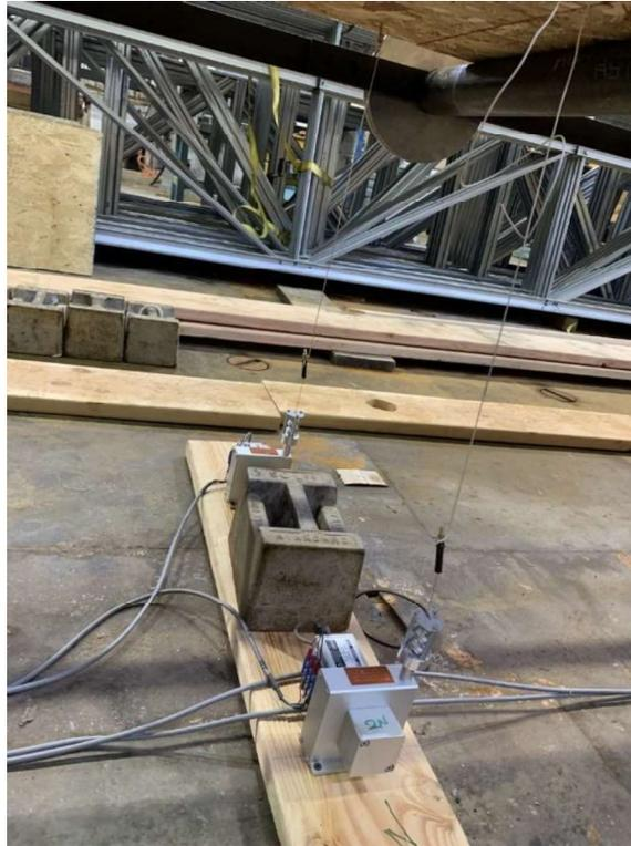
Figure 54: Displacement Potentiometer Placement
