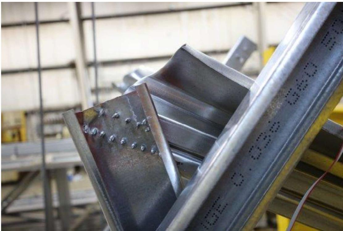
Figure 42: Cutting of Tension Chord Section (AG48-D57)
