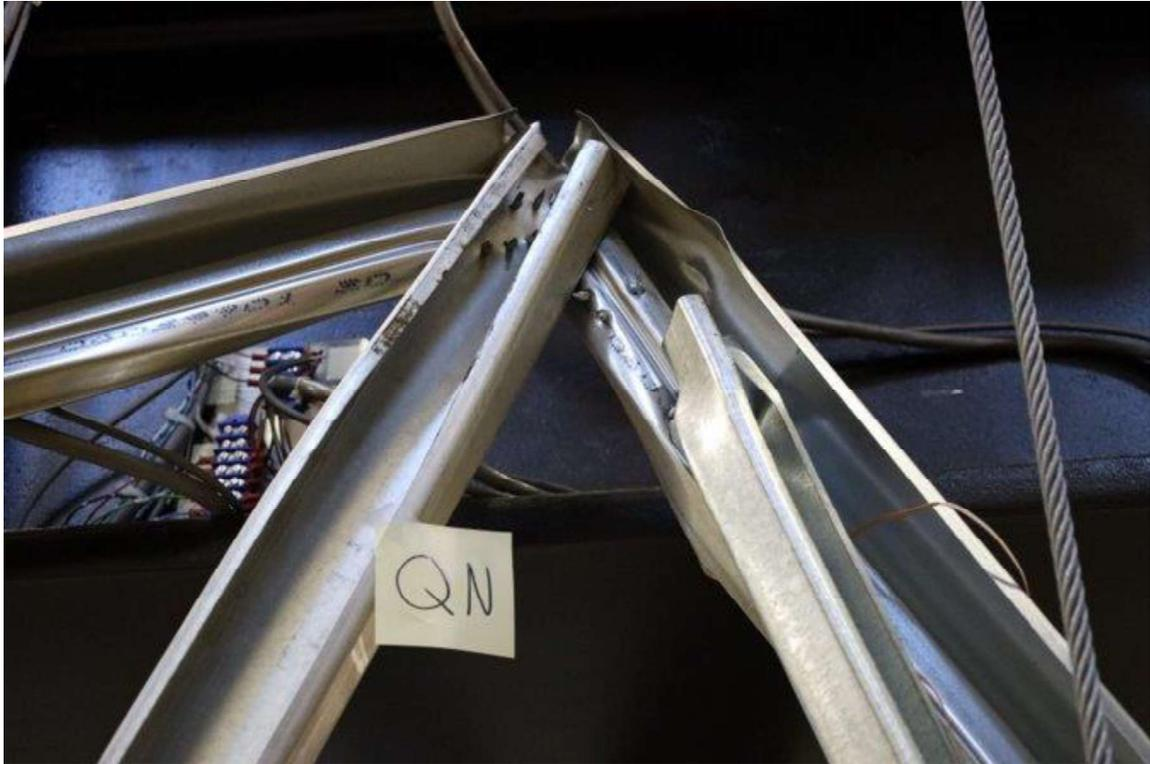
Figure 34: Partial Tearing in Tension Chord at Joint QN (AG48-D35)
