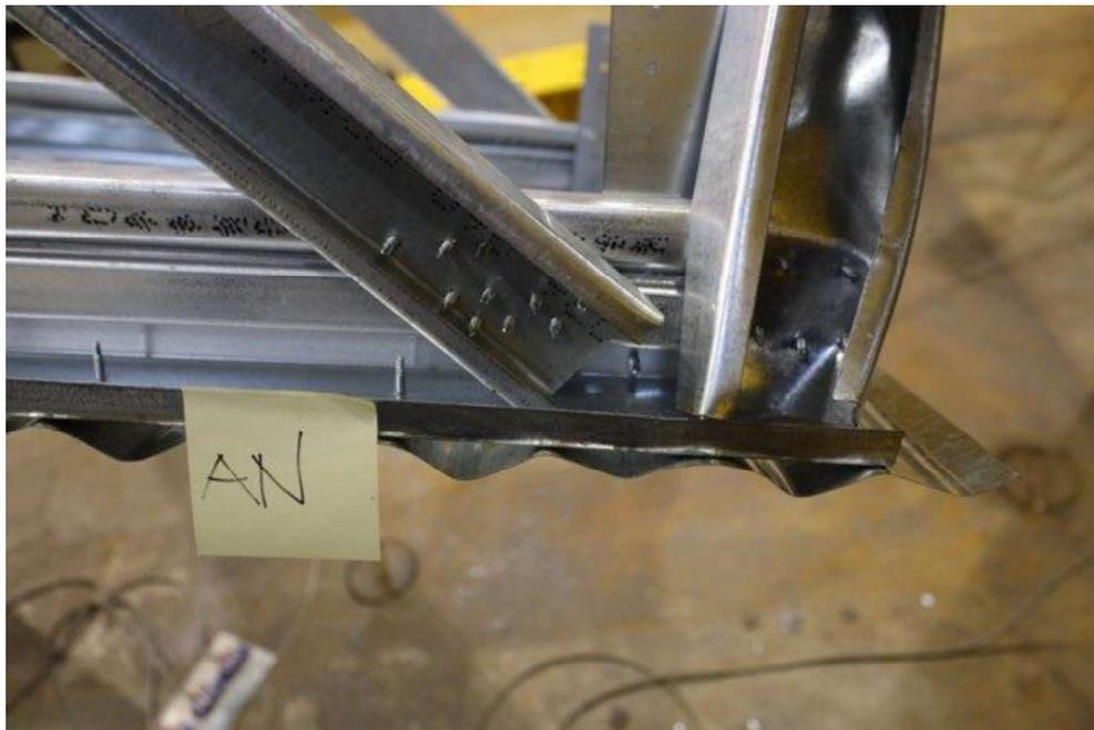
Figure 26: Partial Failures in Web Element Connections (AG36-D35)
