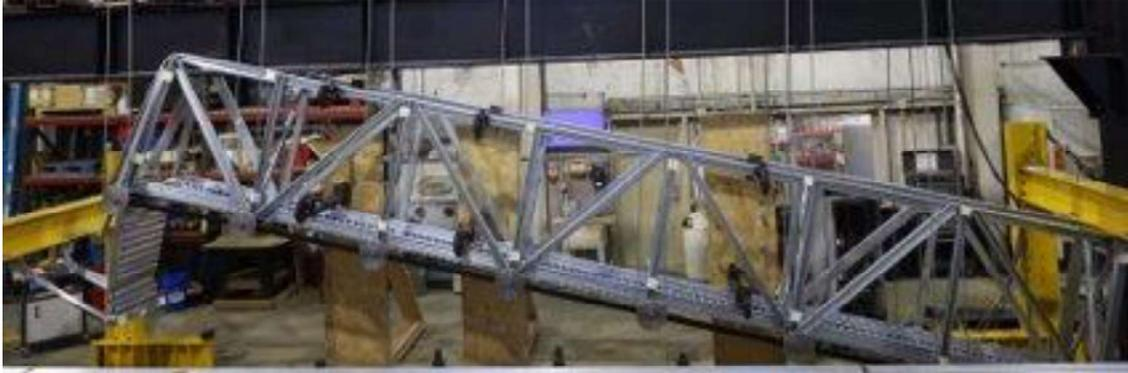
Figure 30: Global Failure of Specimen (AG48-D35)
