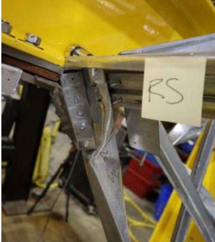
Figure 28: Bearing Connection at Joint RS (AG36-D35)
