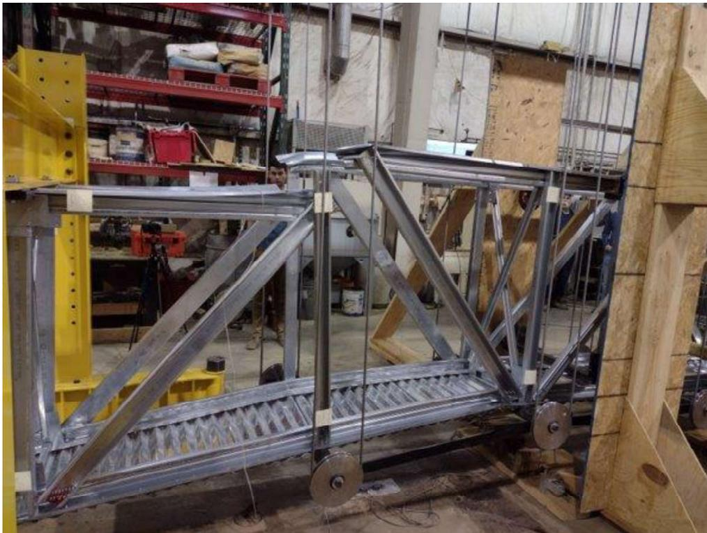
Figure 41: Full Tension Chord Separation
