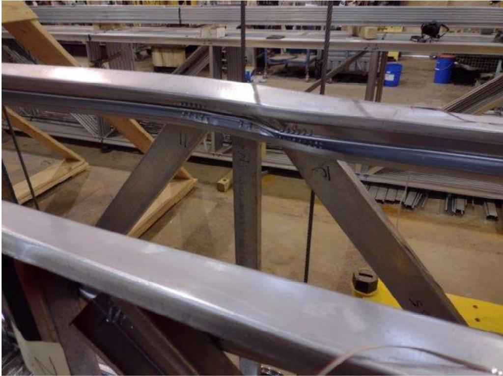
Figure 39: Initial Tension Chord Deformation (AG48-D57)
